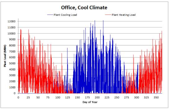
Figure 3. Building with Poor Het Recovery Potential
