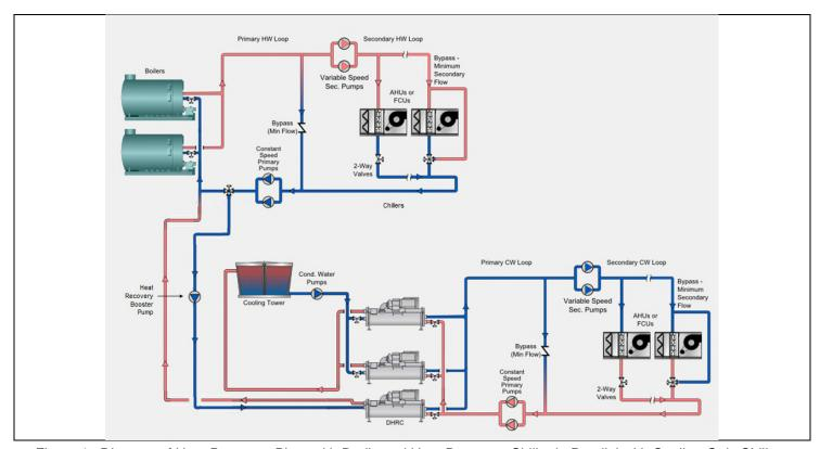
Figure 1. Diagram of Heat Recovery Plant with Dedicated Heat Recovery Chiller in Parallel with Cooling-Only Chillers (Note: This is a simplified diagram only intended to show the basic arrangement of components)
