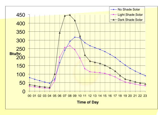
Figure 2 – Hourly Air System Design Load: July, East Exposure
