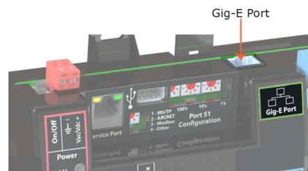
**Fig. 12 – Ethernet Connection Port**
