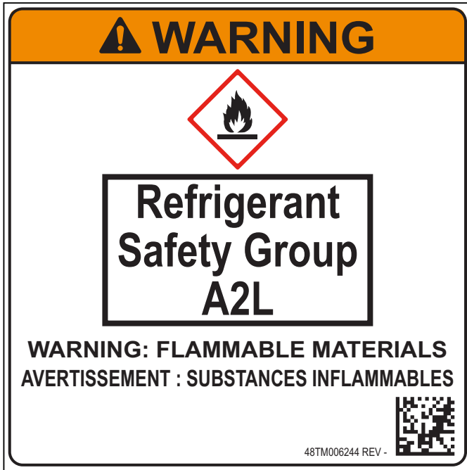
Fig. 63 — A2L Refrigerant Safety Group Warning Label
