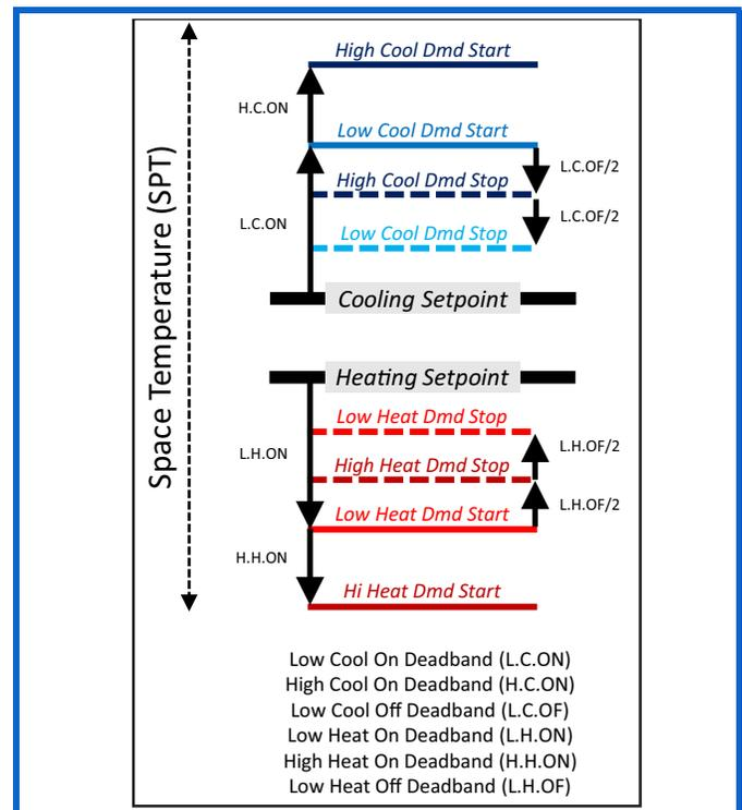
A cool demand is established when the space temperature is above the space temperature setpoint plus the applicable deadband. A heat demand is established when the space temperature is below the space temperature setpoint minus the applicable deadband. Below is a summary of available demands, demand determination, and supply air temperature setpoints for the SPT demand source:
