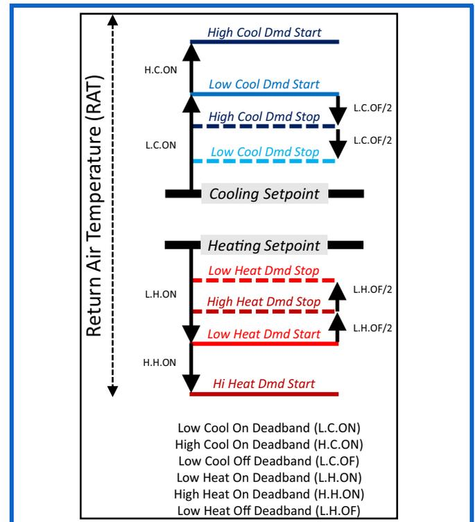
During the occupied period, the control compares the return air temperature to the occupied heating setpoint and applicable deadbands to establish a VAV cool demand. During the unoccupied period, the control compares the return air temperature to the unoccupied cooling setpoint plus applicable deadbands to establish a low or high cool demand.
