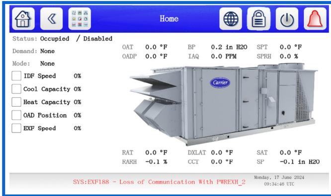
The control navigation is user-friendly with icon-based navigation and descriptive point and property names. Menus and settings are protected by multiple levels of access control, with user level access allowing equipment setup and start-up capability.
