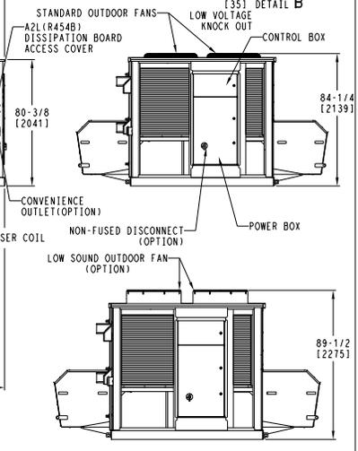
VERTICAL SUPPLY/RETURN - NO RELIEF, BAROMETRIC RELIEF, STD STATIC EXHAUST FAN, MED/HIGH STATIC RETURN FAN
