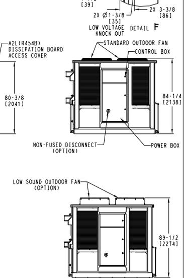
**VERTICAL SUPPLY/RETURN - MED STATIC EXHAUST FAN**
