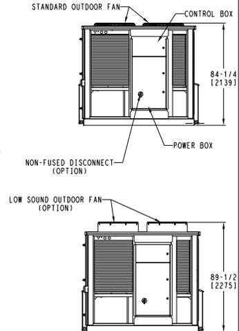
**VERTICAL SUPPLY/RETURN - MED STATIC EXHAUST FAN**
