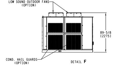
**VERTICAL SUPPLY/RETURN - MED STATIC EXHAUST FAN**
