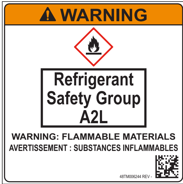
Fig. 65 — A2L Refrigerant Safety Group Warning Label
