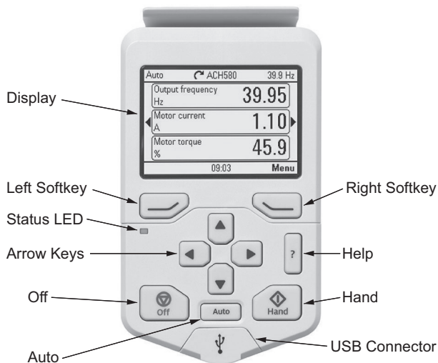
Fig. 40 — ACH580 VFD Keypad — Front
