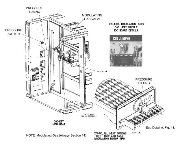
Fig. 43 — Modulating Gas Heat
