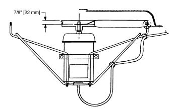
Fig. 53 — Condenser-Fan Adjustment
