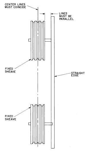
Fig. 52 — Pulley Alignment
