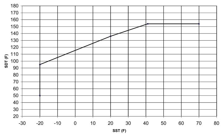
Fig. 17 — High Pressure/SCT Alarm Upper Envelope
