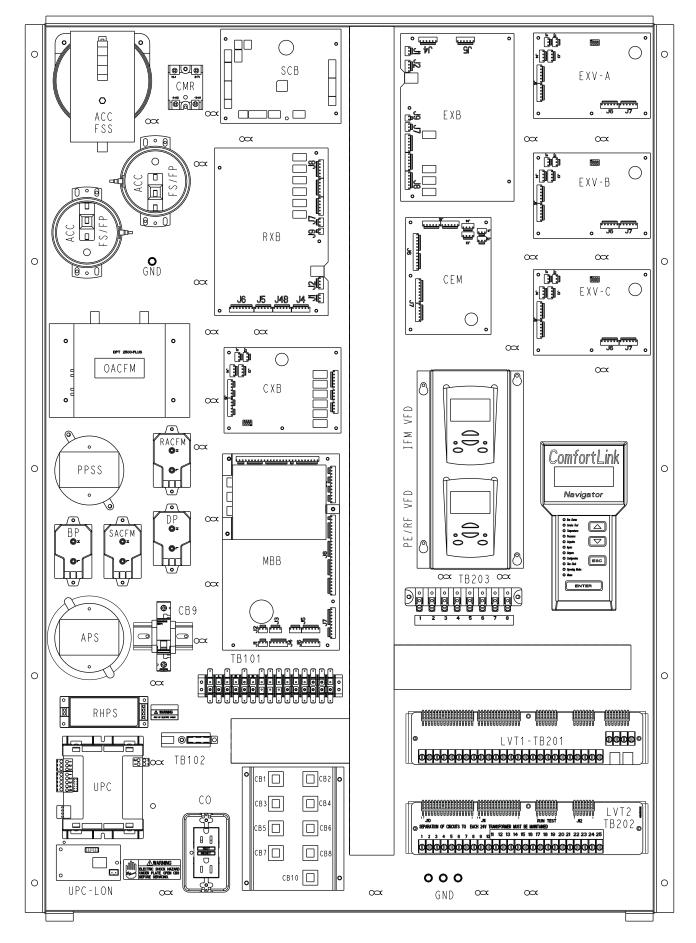
Fig. 31 — 48/50N Component Arrangement Control Box
