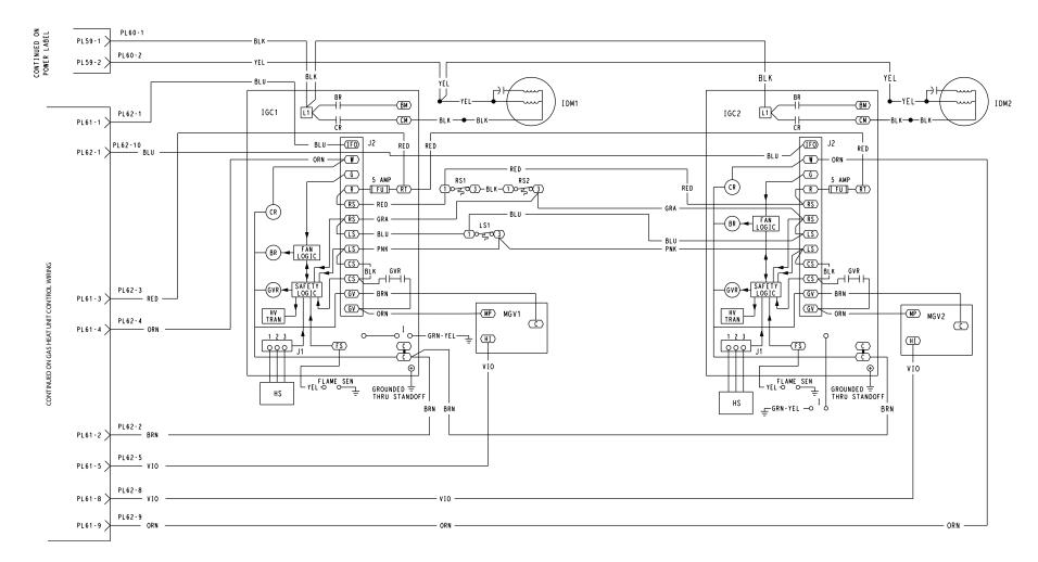
Fig. 25 — 48N Typical Gas Heat Section Wiring (Nominal Ton 75 to 105, Low Heat Units)
