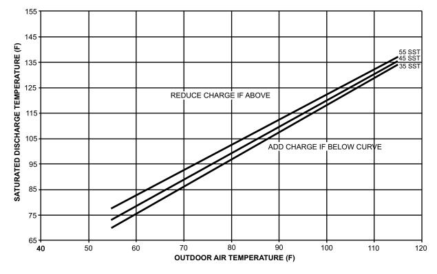
Fig. 67 — Charging Chart — 105 Ton High Capacity, High Efficiency
