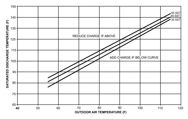
Fig. 62 — Charging Chart — 90 Ton High Capacity, Standard Efficiency
