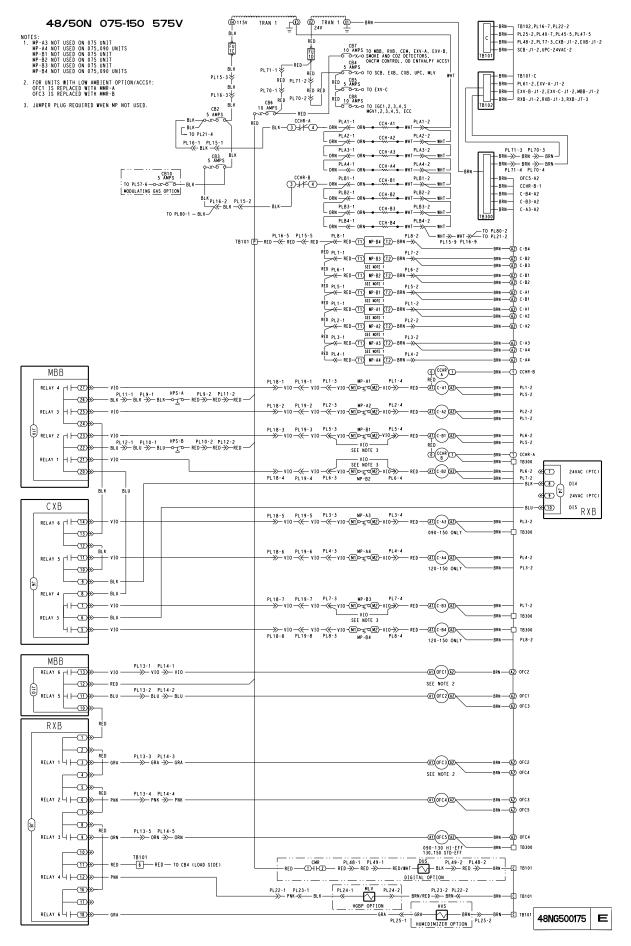
Fig. 29 — 48/50N Component Control Wiring, 575 v (Nominal Ton 075 to 150 Units)
