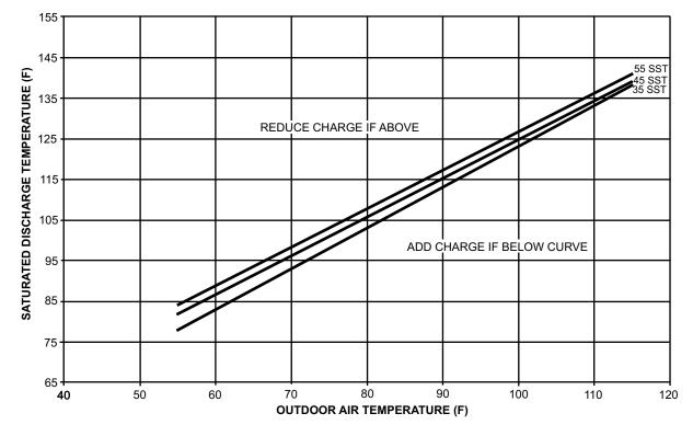
Fig. 75 — Charging Chart — 130 Ton High Capacity, High Efficiency
