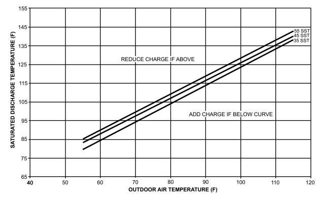
Fig. 73 — Charging Chart — 130 Ton Standard Capacity, High Efficiency
