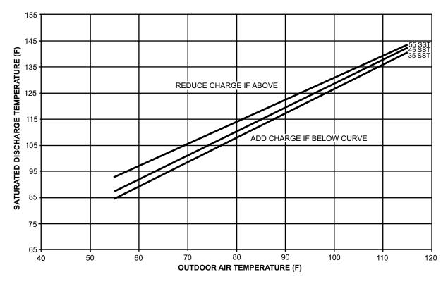
Fig. 58 — Charging Chart — 75 Ton High Capacity, Standard Efficiency
