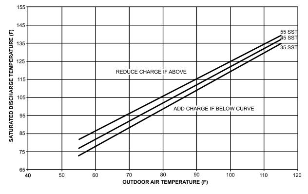
Fig. 57 — Charging Chart — 75 Ton Standard Capacity, High Efficiency
