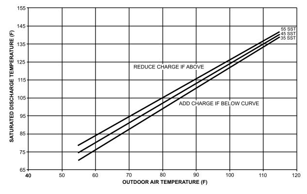
Fig. 59 — Charging Chart — 75 Ton High Capacity, High Efficiency
