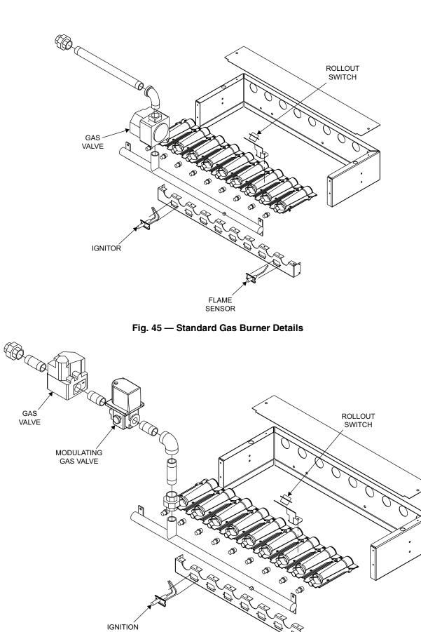
Fig. 46 — Modulating Gas Burner Assembly
