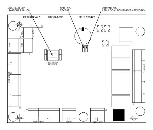
Fig. 34 — Staged Gas Heat Control Board (SCB)
