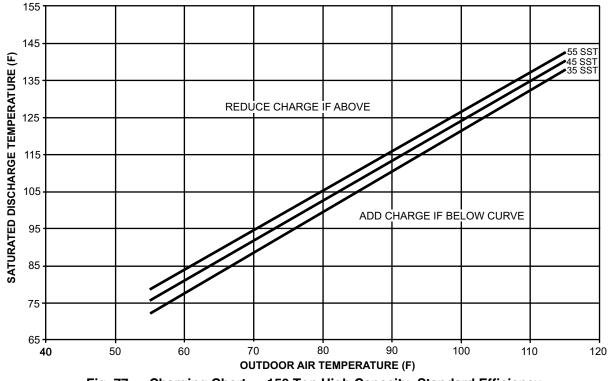
Fig. 77 — Charging Chart — 150 Ton High Capacity, Standard Efficiency
