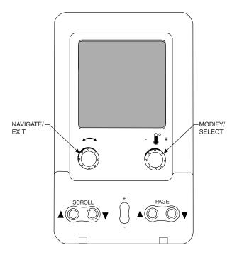
Fig. 2 — System Pilot User Interface
