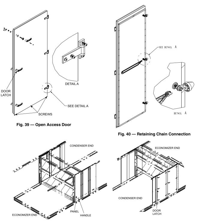
Fig. 41 — Additional Access Panel Removal
