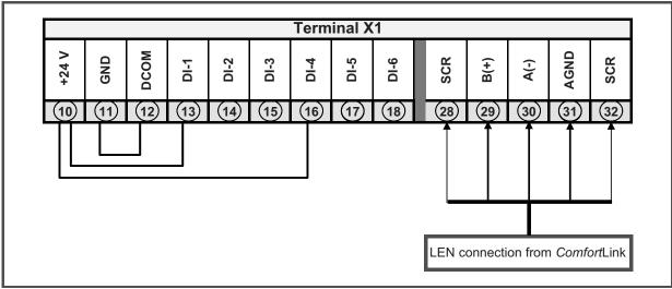
Fig. 38 — VFD Wiring
