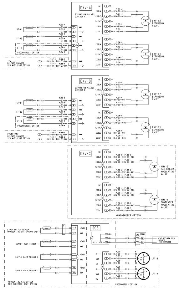
Fig. 22 — 48/50N EXV, SCB Input/Output Connections
