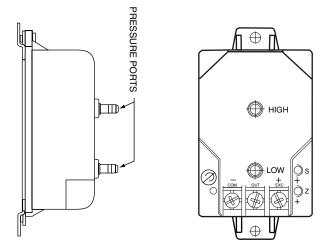
Fig. 55 — Transducer Details
