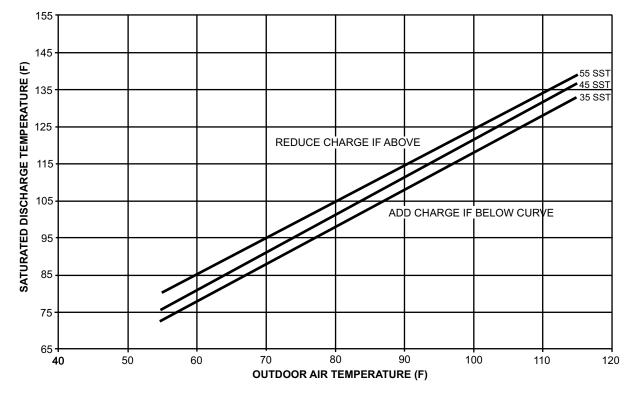
Fig. 65 — Charging Chart — 105 Ton Standard Capacity, High Efficiency
