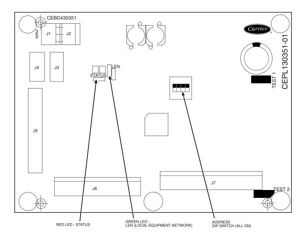
Fig. 35 — Controls Expansion Board (CEM)
