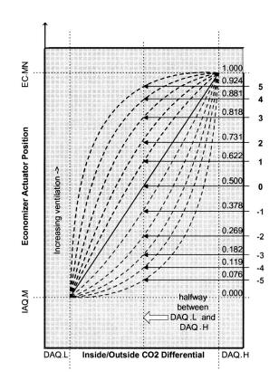
NOTE: Calculating the IAQ.M and EC.MN damper position based on differential IAQ measurement.
