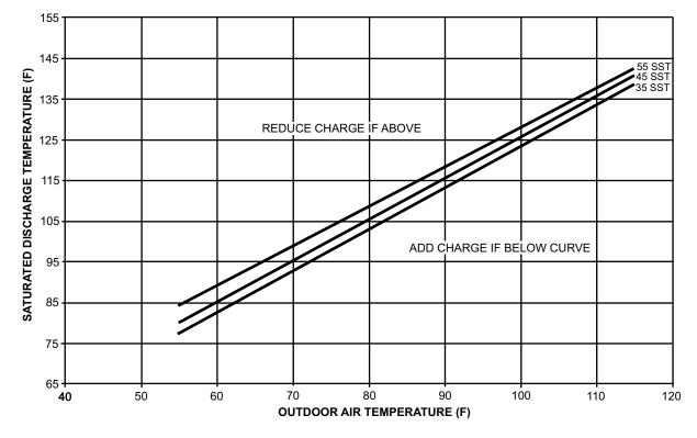
Fig. 71 — Charging Chart — 120 Ton High Capacity, High Efficiency
