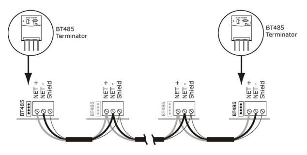
Fig. K — Network Wiring
