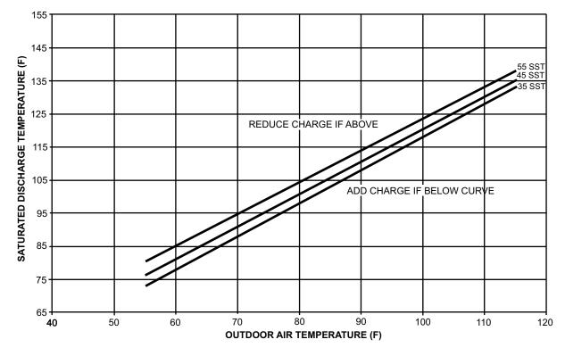
Fig. 63 — Charging Chart — 90 Ton High Capacity, High Efficiency
