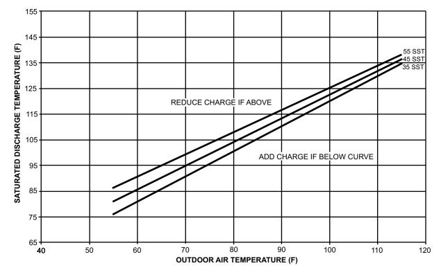
Fig. 69 — Charging Chart — 120 Ton Standard Capacity, High Efficiency
