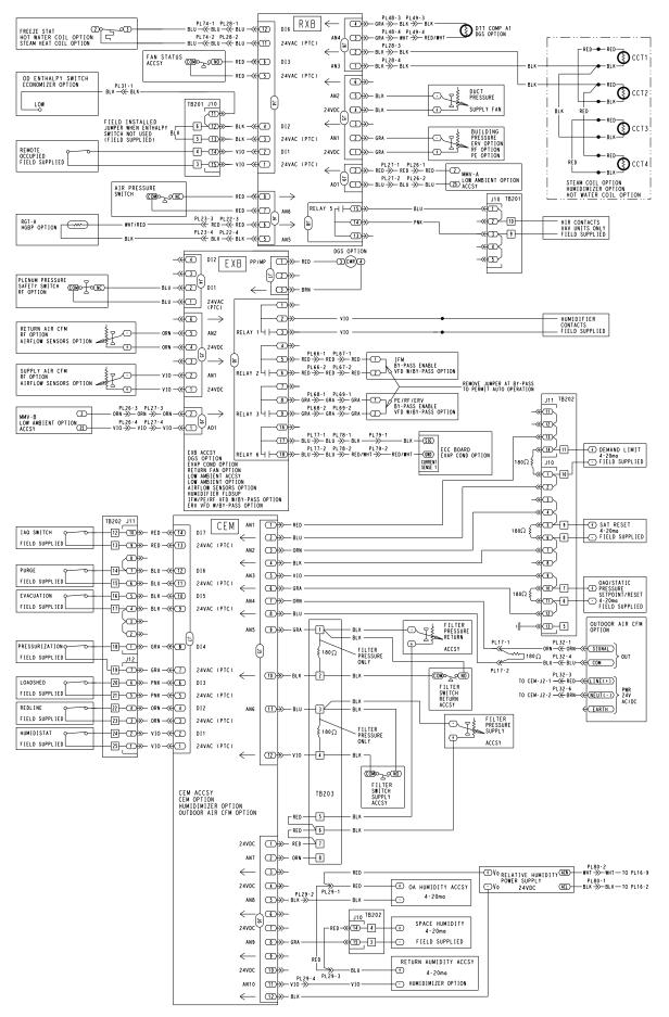
Fig. 21 — 48/50N RXB, EXB, CEM Input/Output Connections
