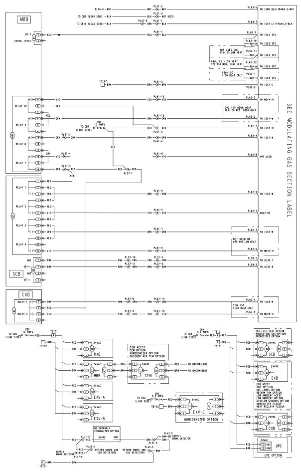
Fig. 23 — 48N Typical Modulating Gas Heat Unit Control Wiring
