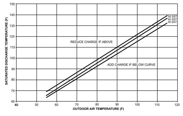
Fig. 61 — Charging Chart — 90 Ton Standard Capacity, High Efficiency
