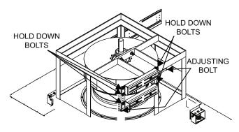
Fig. 49 — Return Fan Motor Plate Adjustment
