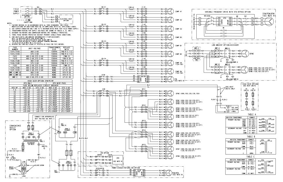
Fig. 19 — 48/50N Typical Power Schematic (Nominal Ton 90-150 Units Shown)
