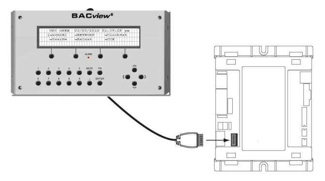
Fig. M — BACview<sup>6</sup> Device Connection
