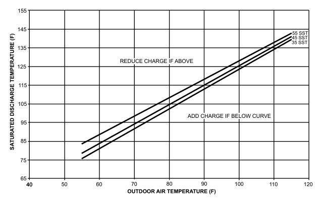
Fig. 74 — Charging Chart — 130 Ton High Capacity, Standard Efficiency
