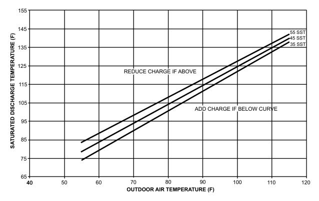
Fig. 66 — Charging Chart — 105 Ton High Capacity, Standard Efficiency
