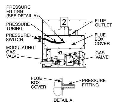
Fig. 44 — Gas Section Detail, Modulating Gas Heat
