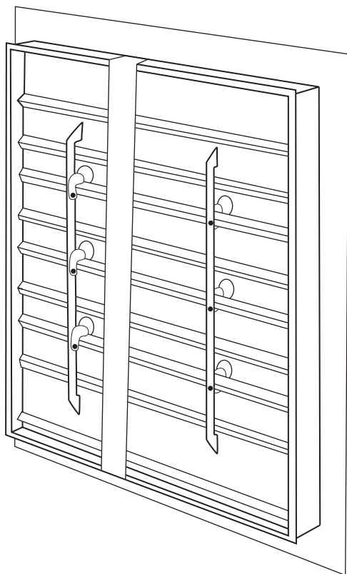
Fig. 18 — Optional Exhaust Damper
