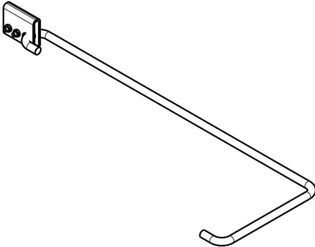
**Fig. 23 — Circuit Breaker Handle Extension**
