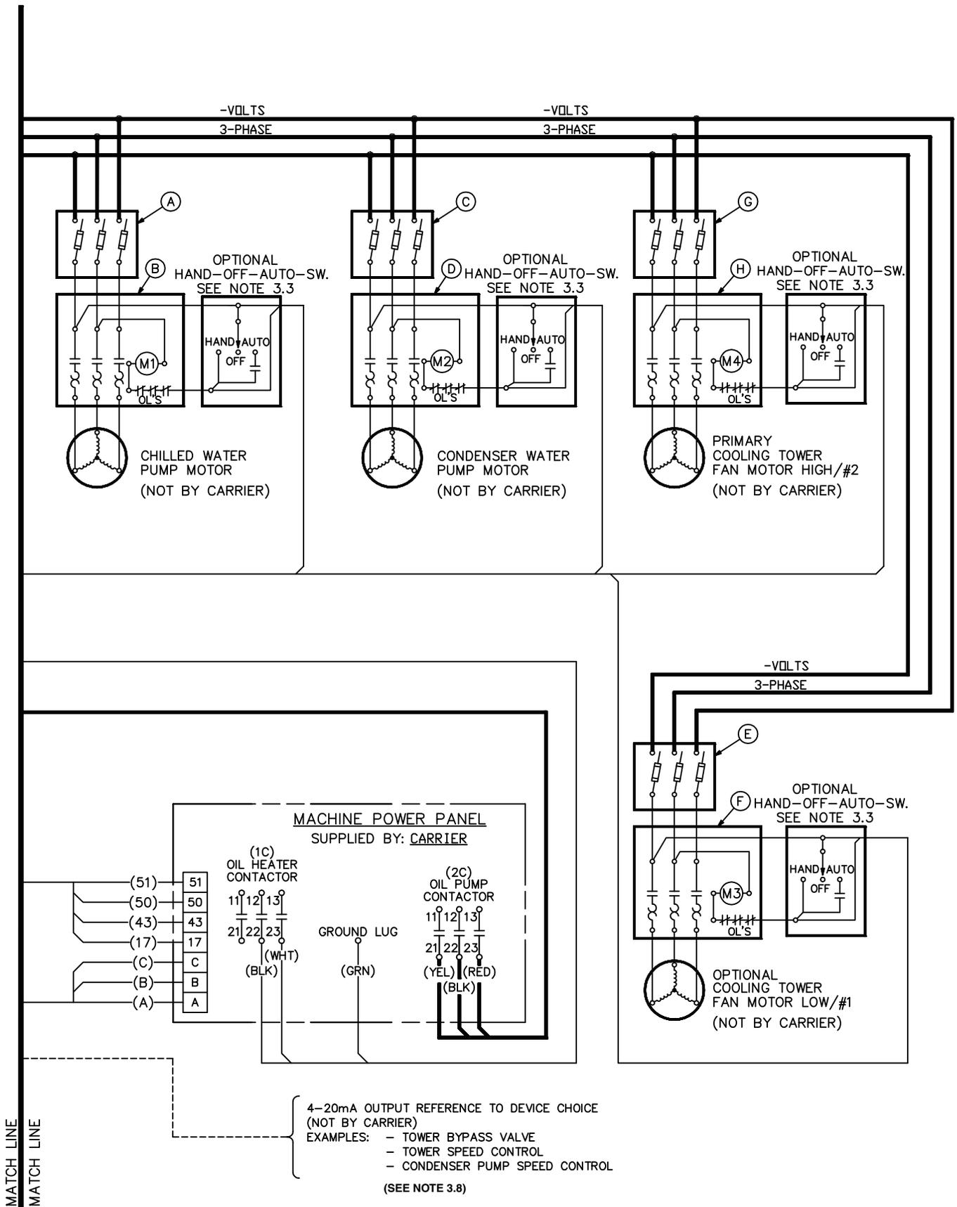
**Fig. 30 — 19XR Typical Field Wiring with Benshaw Free-Standing Starter (Low Voltage) (cont)**
