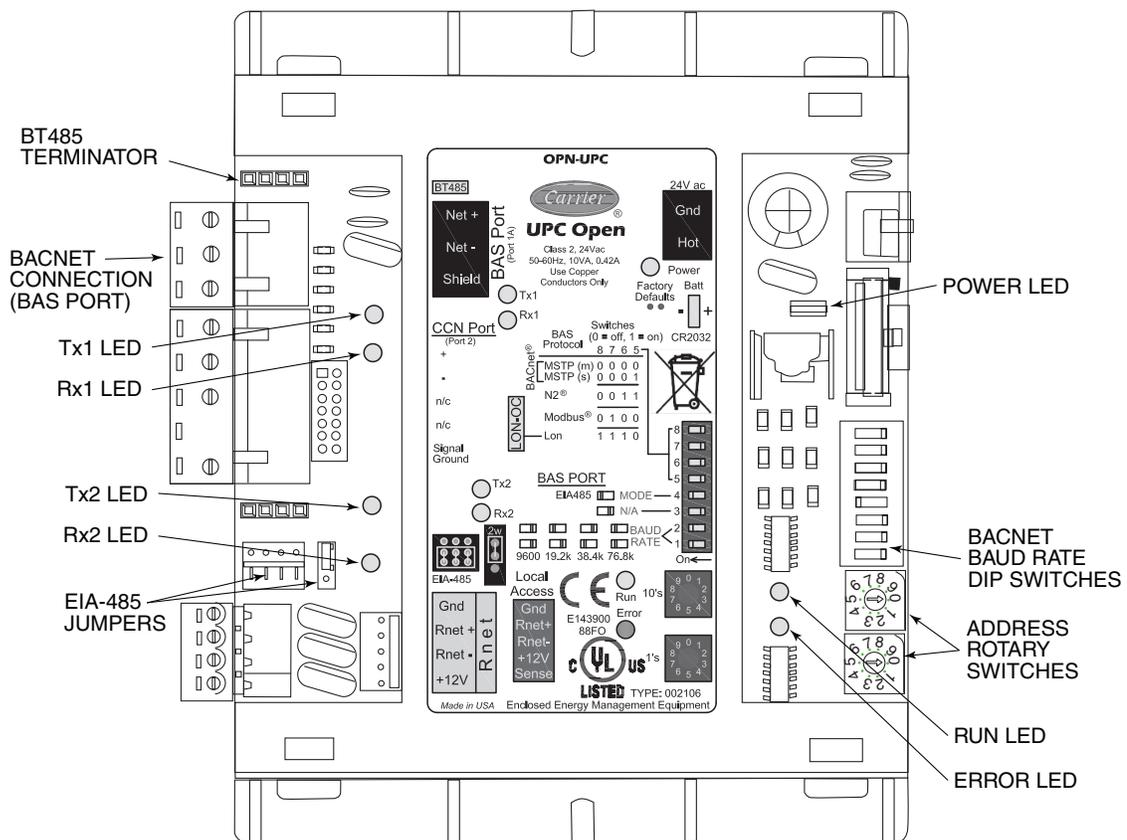
Fig. 37 — UPC Open Controller
