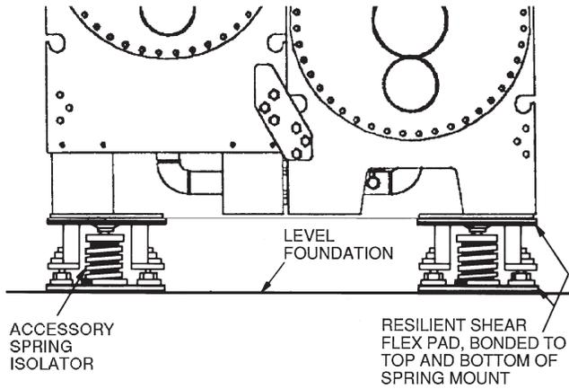
NOTE: The accessory spring isolators are supplied by Carrier for installation in the field.
