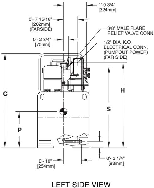
**Fig. 18 — Optional Pumpout Unit and Storage Tank**
