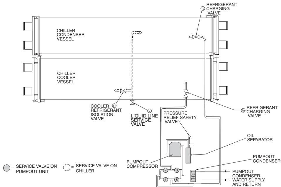
Fig. 20 — Optional Pumpout System Piping Schematic without Storage Tank
