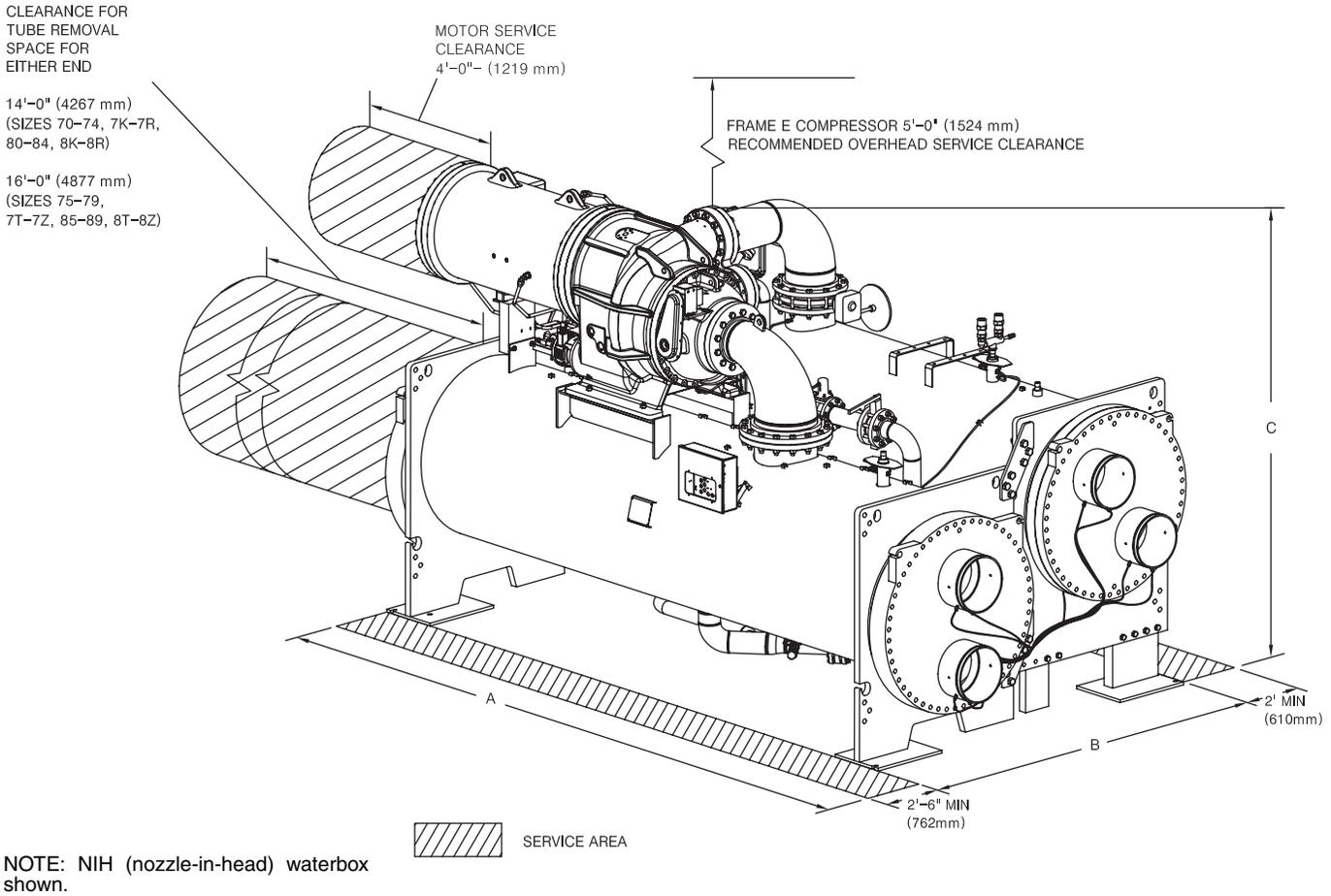
**Fig. 4 — 19XR, XRV Two-Stage Chiller Dimensions**
