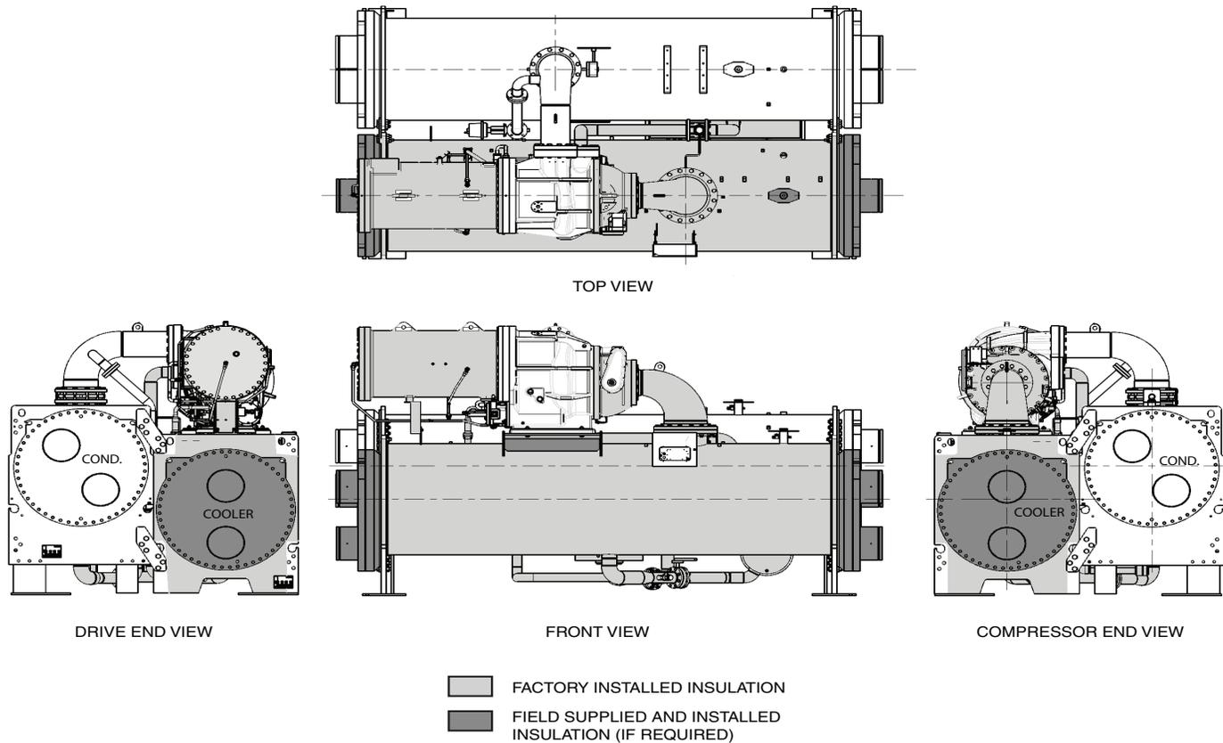
**Fig. 40 — 19XR,XRV Insulation Area**
