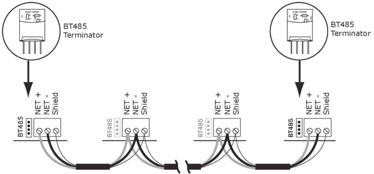
Fig. 38 — Network Wiring
