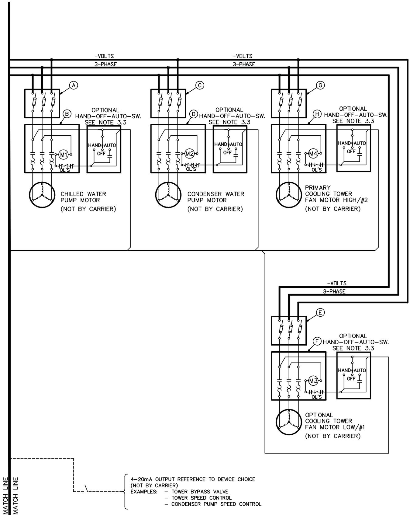
Fig. 28 — 19XR Typical Field Wiring with Unit-Mounted Starter (Benshaw Starter Shown) (cont)
