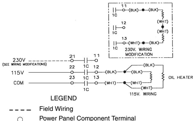
**Fig. 35 — Oil Heater and Control Power Wiring (Units without Split Ring Diffuser)**
