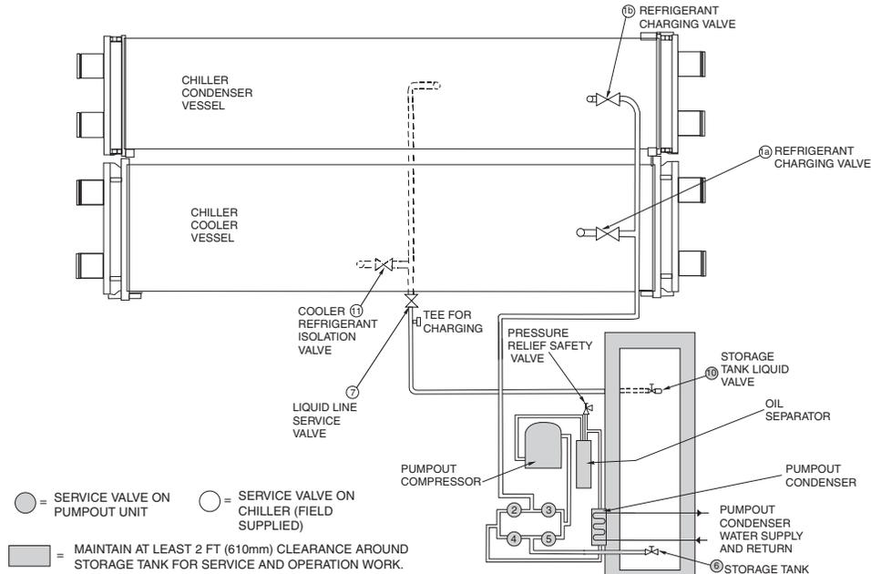
Fig. 19 — Optional Pumpout System Piping Schematic with Storage Tank
