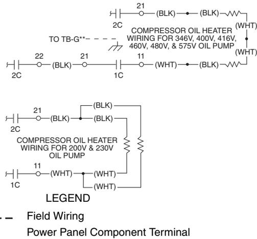
**Fig. 36 — Oil Heater and Control Power Wiring (Units with Split Ring Diffuser)**
