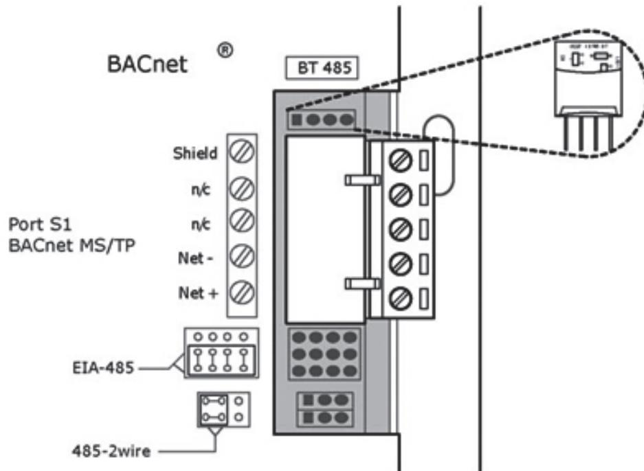
Fig. 39 — BT485 Terminator Installation
