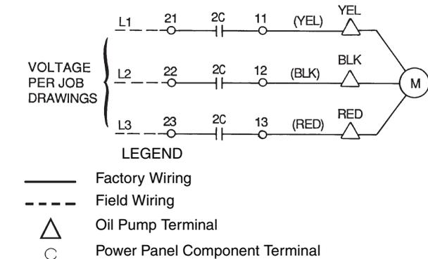
**Fig. 34 — Oil Pump Wiring**
