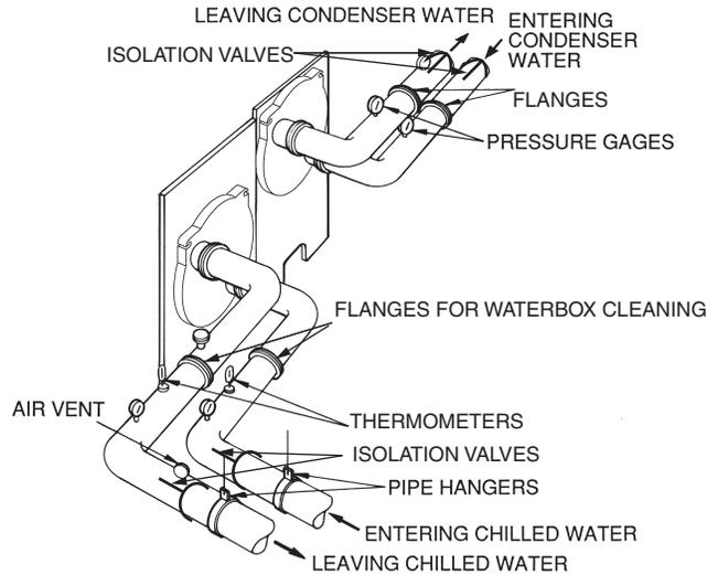
**Fig. 15 — Typical Nozzle Piping**
