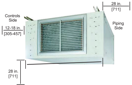
42DF Unit Clearance and Service Access
