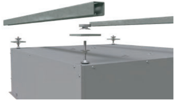
Fig. 58 — Channel Mount Suspension (42CK Units)
