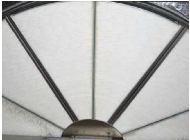
Fig. 35 — Embedded Stiffener Facing Motor Side
