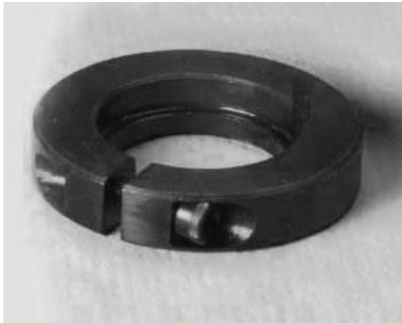
Fig. 7 — Tightening Locking Collar
