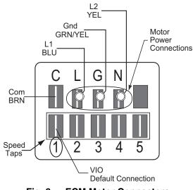
Fig. 6 — ECM Motor Connectors
