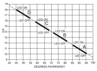
Fig. 60 — Outside Air Temperature Changeover Set Points
