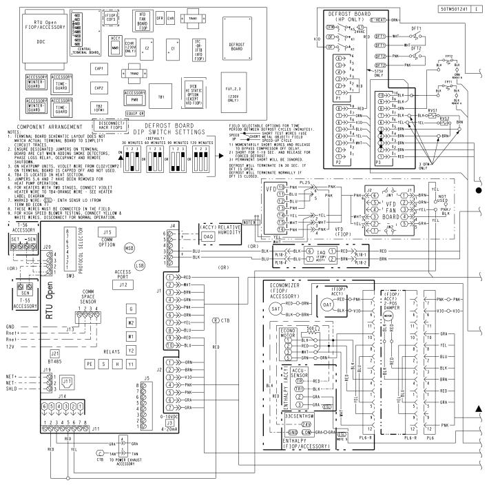
Fig. 53 — RTU Open Overlay for Economizer Wiring
