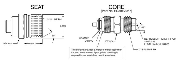
Fig. 18 — CoreMax<sup>1</sup> Access Port Assembly
