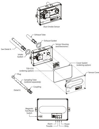
Fig. 40 — Smoke Detector Sensor
