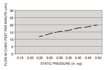
Fig. 61 — Outdoor-Air Damper Leakage
