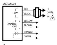
POWER SUPPLY. PROVIDE DISCONNECT MEANS AND OVERLOAD PROTECTION AS REQUIRED.
