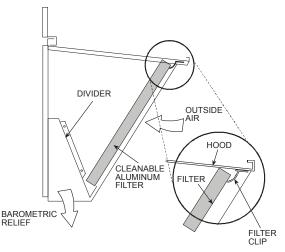
Fig. 3 — Filter Installation
