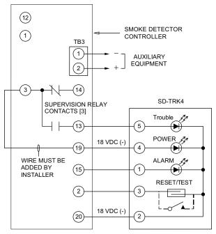
Fig. 47 — Remote Test/Reset Station Connections
