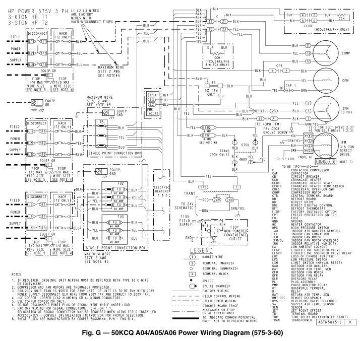
Fig. G — 50KCQ A04/A05/A06 Power Wiring Diagram (575-3-60)
