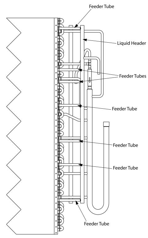
NOTE: In heating mode, the liquid header on the condenser coil has Accutrol in each feeder tube.
