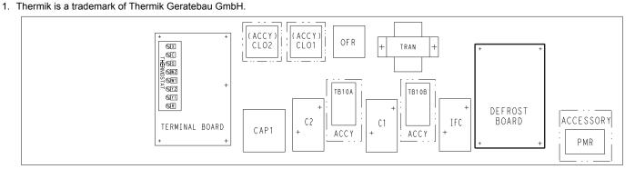
Fig. 28 — Defrost Control Board Location
