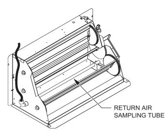
Fig. 43 — Return-Air Sampling Tube Location
