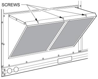
Fig. 4 — Screens Installed on Outdoor-Air Hood
