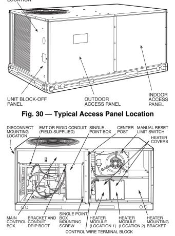
Fig. 31 — Typical Component Location
