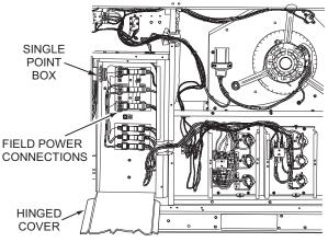
Fig. 33 — Typical Single Point Installation
