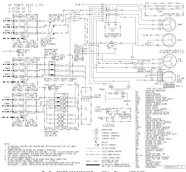
Fig. F — 50KCQ A04/A05/A06 Power Wiring Diagram (460-3-60)
