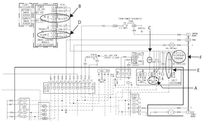
Fig. 46 — Typical Smoke Detector Wiring
