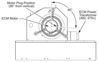
Fig. 5 — 50KCQ Direct-Drive Supply Fan Assembly
