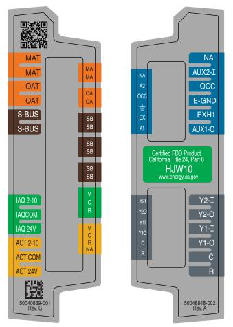
Fig. 67 — W7220 Wiring Terminals
