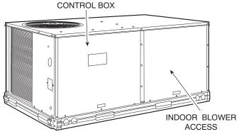
Fig. 1 — Typical Access Panel Location (Front)
