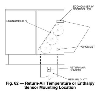
In this mode of operation, the outdoor-air temperature is compared to the return-air temperature and the lower temperature airstream is used for cooling. When using this mode of changeover control, turn the enthalpy set point potentiometer fully clockwise to the D setting. (See Fig. 59.)
