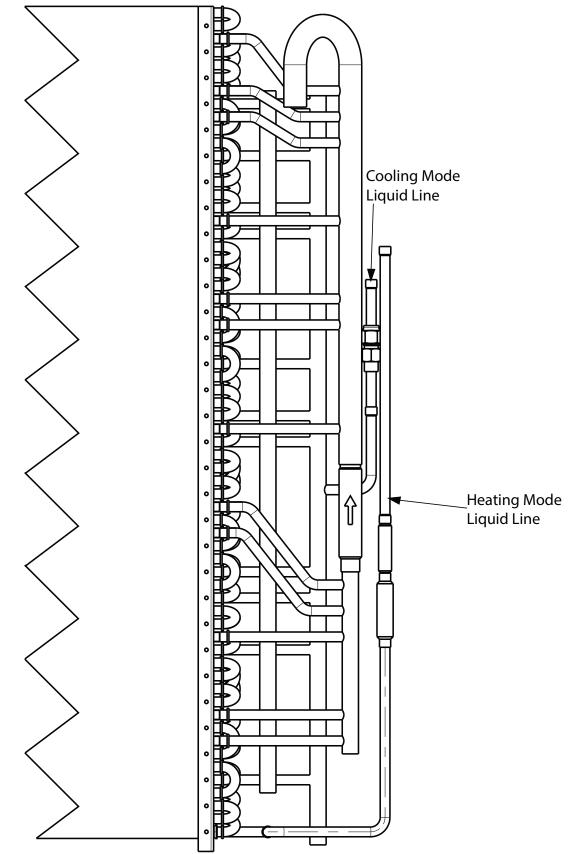
NOTE: While in cooling mode, the liquid line header has Accutrol in each feeder tube.
