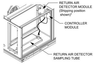
\*RA detector must be moved from shipping position to operating position by installer.
