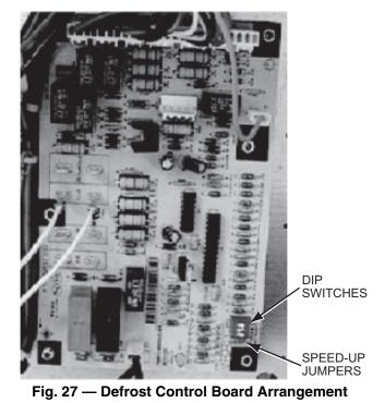
The DFB is located in the 50KCQ's main control box (see Fig. 28). All connections are factory-made through harnesses to the unit's CTB, to IFC (belt-drive motor) or to ECM (direct-drive motor), reversing valve solenoids and to defrost thermo-stats. Refer to Table 8 for details of DFB Inputs and Outputs. Detailed unit operating sequences are provided in the Start-Up section starting on page 55.
