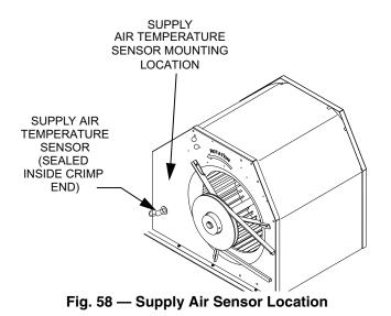
The temperature sensor looks like an eyelet terminal with wires running to it. The sensor is located in the "crimp end" and is sealed from moisture.
