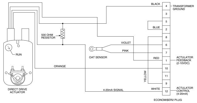
Fig. 56 — EconoMi\$er2 with 4 to 20 mA Control Wiring
