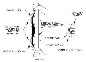
Fig. 10 — Supply-Fan Pulley Adjustment
