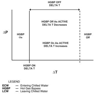
$<sup>\</sup>Delta P$  = (Condenser Pressure) – (Cooler Pressure)  $\Delta T$  = (ECW) – (LCW)
