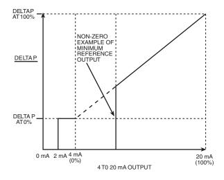
Fig. 29 — Head Pressure Reference Output
