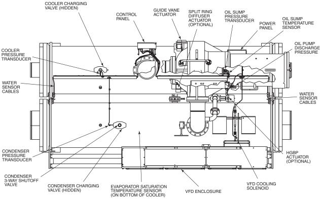
Fig. 12 — Chiller Controls and Sensor Locations
