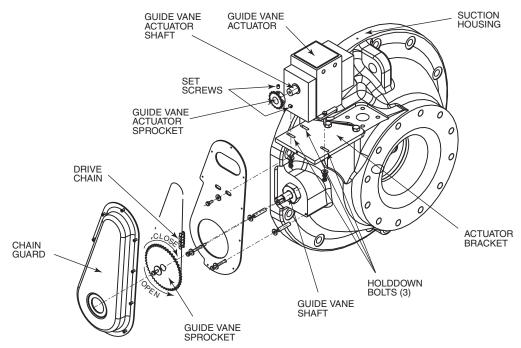
Fig. 50 — Guide Vane Actuator Linkage
