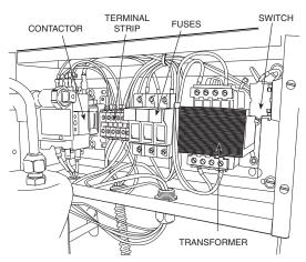
Fig. 54 — Pumpout Control Box (Interior)
