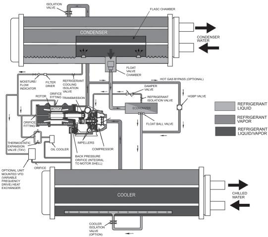
Fig. 5 — Refrigeration Cycle — 19XRV Two-Stage Compressor
