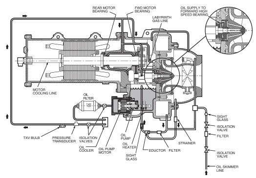
Fig. 6 — Single-Stage Lubrication System
