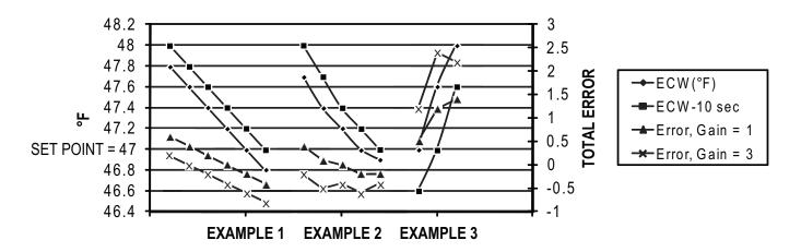
Fig. 25 — Transient Example of ECW Gain
