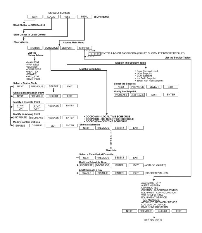
Fig. 20 — 19XRV Chiller Display Menu Structure (ICVC Version 9)
