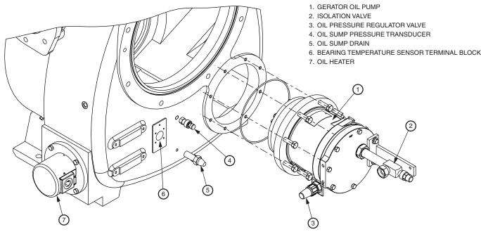
Fig. 8 — Gerotor Oil Pump
