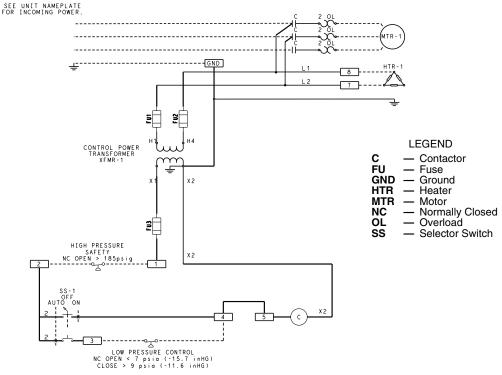
Fig. 48 — Pumpout Unit Wiring Schematic
