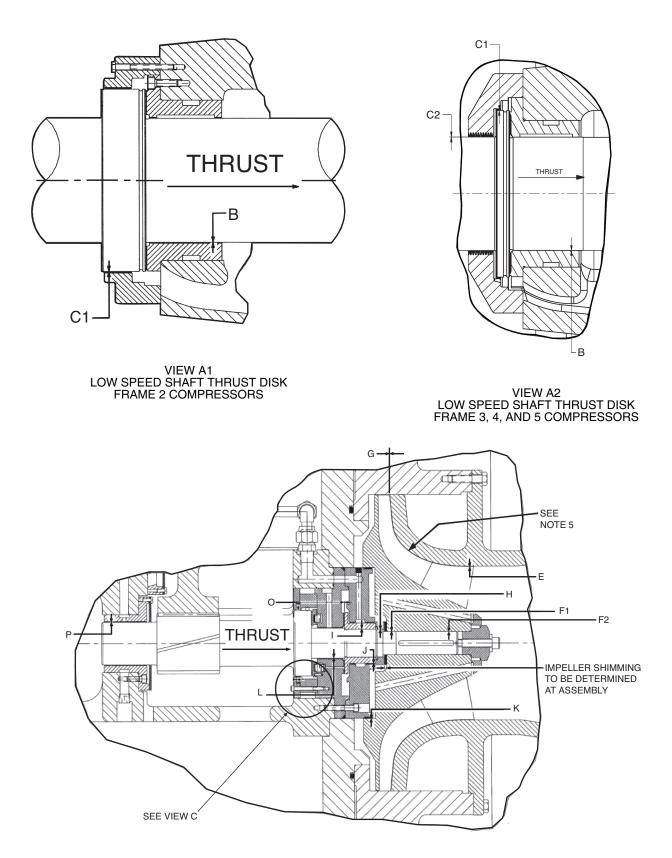
VIEW B — HIGH SPEED SHAFT, ORIGINAL DESIGN (OIL FILM BEARINGS) AND IMPELLER SECTION
