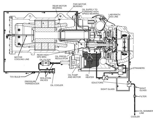
Fig. 7 — Two-Stage Lubrication System
