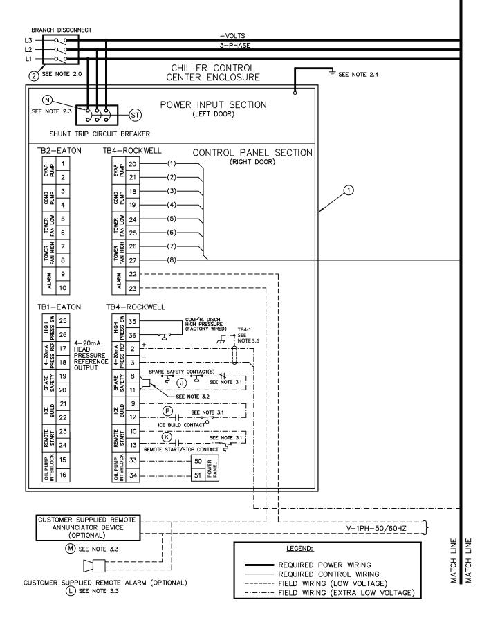
Fig. 70 — 19XRV Field Wiring — Standard Tier VFD
