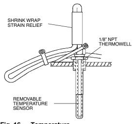
Fig. 16 — Temperature Sensor Used
