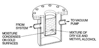
Fig. 37 — Dehydration Cold Trap
