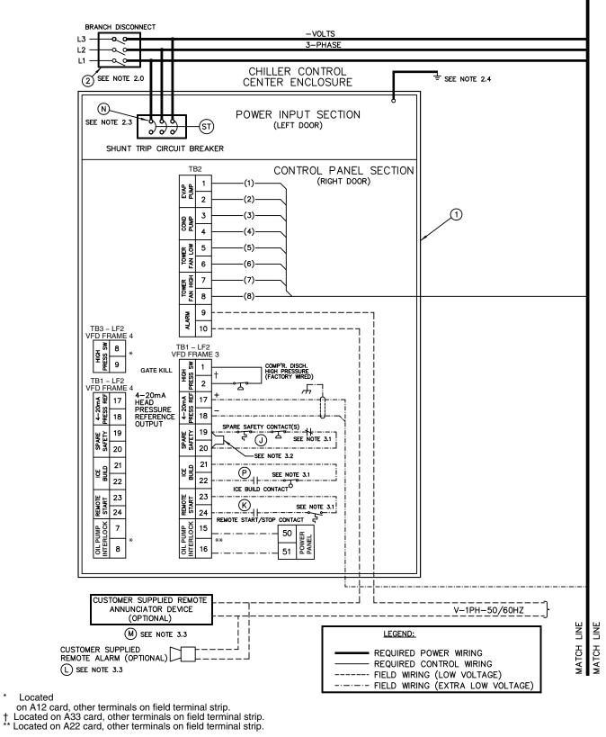
Fig. 69 — 19XRV Field Wiring — LiquiFlo<sup>™</sup> 2 VFD
