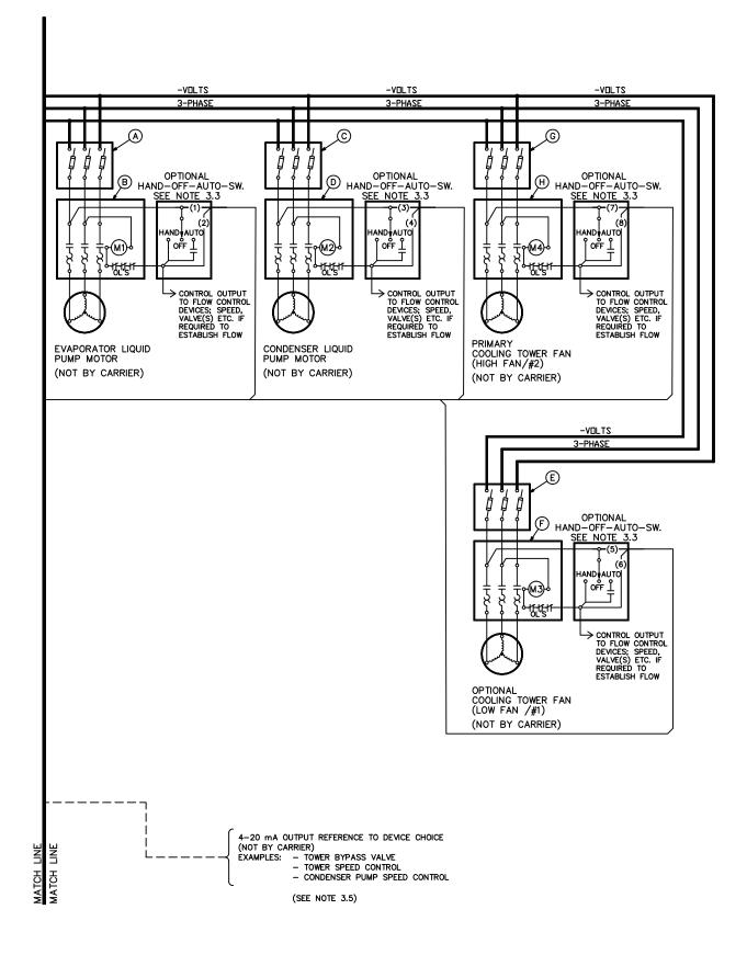
Fig. 70 — 19XRV Field Wiring — Standard Tier VFD (cont)
