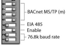
Fig. C — DIP Switches
