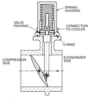
Fig. 53 — Economizer Damper Valve (Two-Stage Compressor Chiller)
