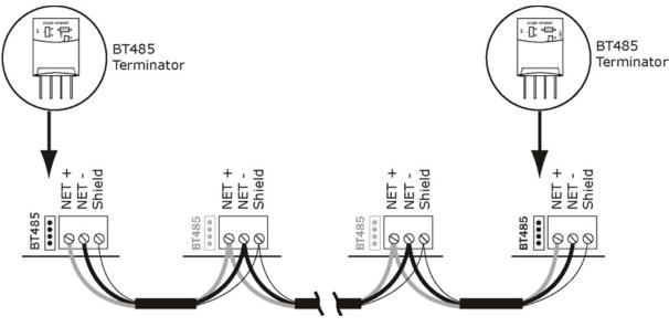
Fig. D — Network Wiring
