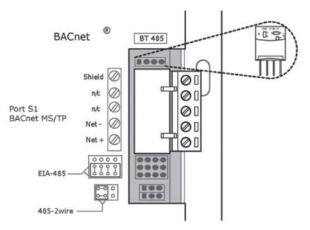
Fig. E — BT485 Terminator Installation
