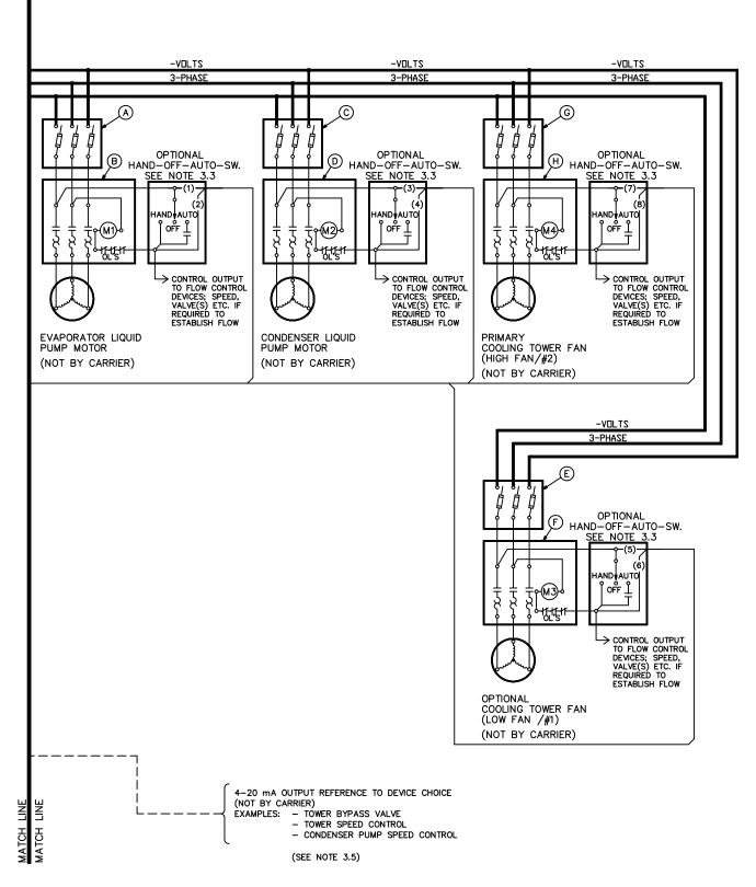
Fig. 69 — 19XRV Field Wiring — LiquiFlo<sup>™</sup> 2 VFD (cont)
