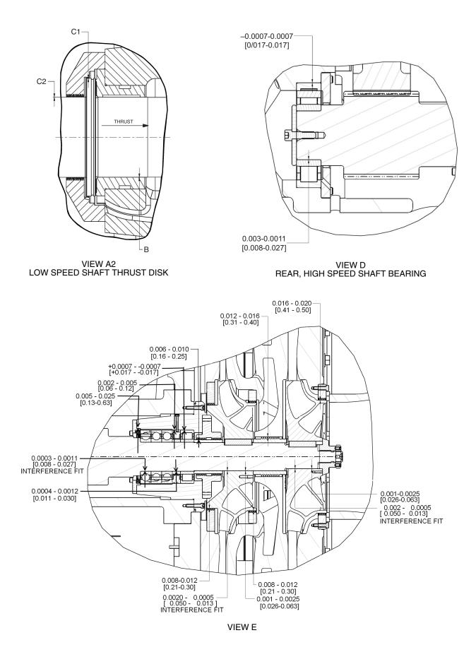
Fig. 60 — Compressor Fits and Clearances — Two-Stage Compressors (cont)
