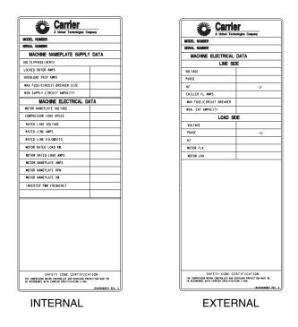
Fig. 40 — Machine Electrical Data Nameplate
