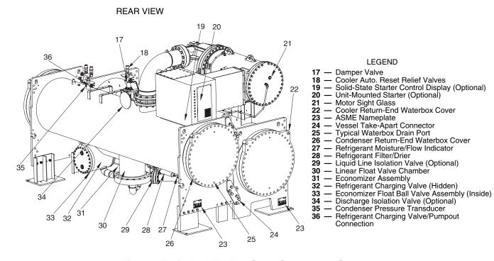
Fig. 3 — Typical 19XRV Two-Stage Compressor Components
