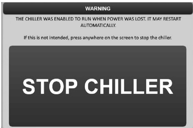
Fig. 36 — Chiller May Restart Automatically Warning Screen
