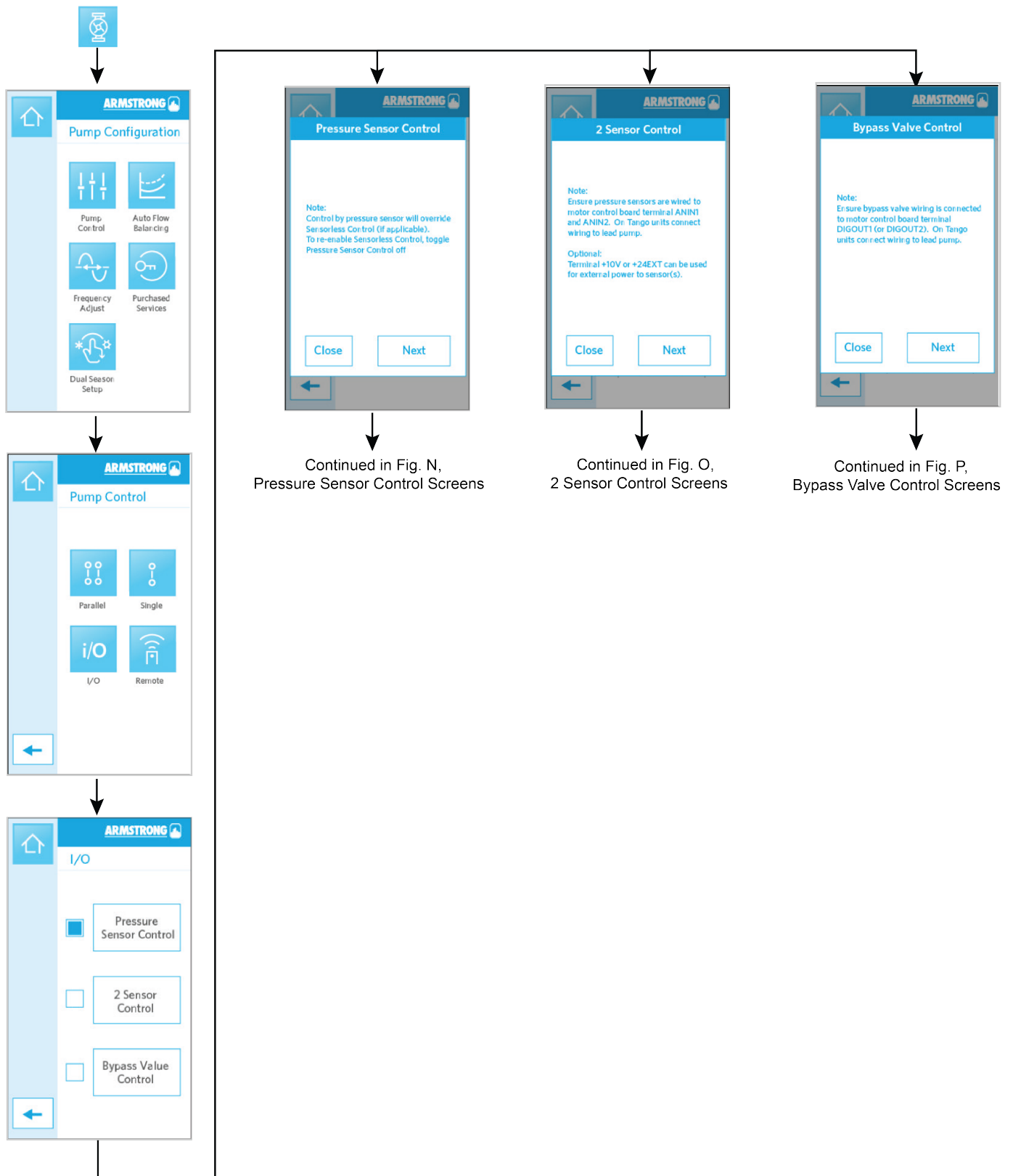
Fig. M — Sensor and Bypass Valve Control Screens
