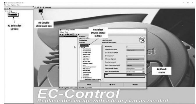
Fig. 21 – EC-Control Fan Connection Verification
