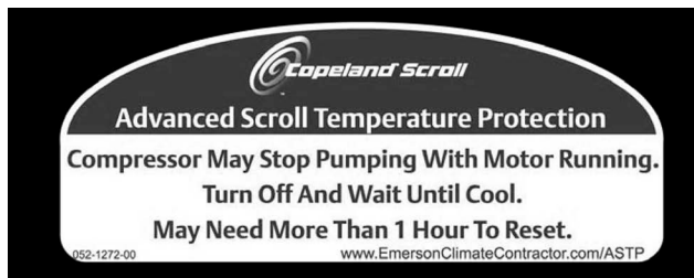
Fig. 4 — Advanced Scroll Temperature Protection Label
