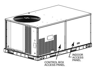
Fig. 33 — Typical Access Panel Location
