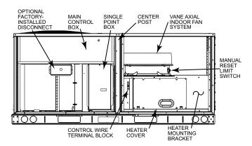
Fig. 34 — Typical Component Location
