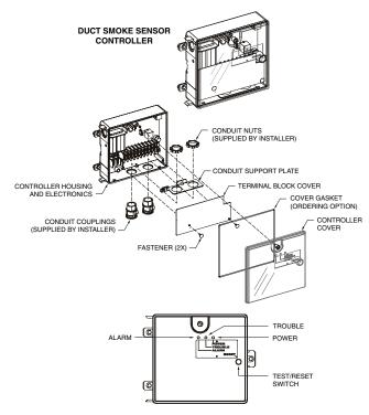
Fig. 39 — Controller Assembly
