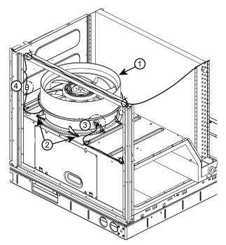
Fig. 14 — Fan Assembly Install
