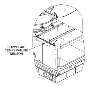
Fig. 59 — Supply Air Sensor Location
