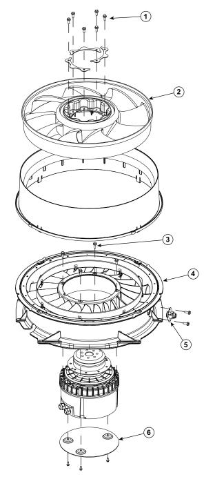
Fig. 12 — Disassembling Motor and Fan Assembly
