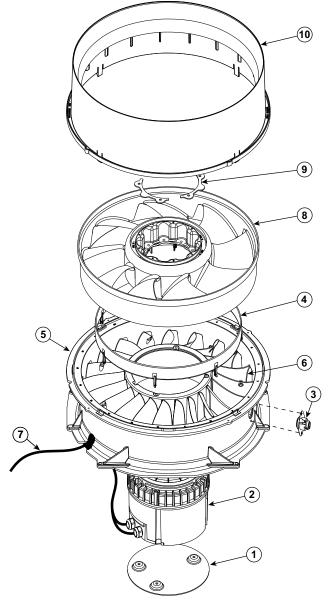
Fig. 13 — Fan System Re-Assembly
