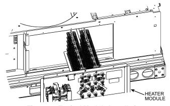
Fig. 35 — Typical Module Installation
