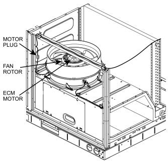
Fig. 5 — Direct-Drive Supply Fan Assembly
