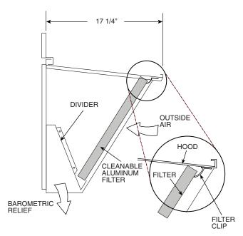
Fig. 3 — Filter Installation
