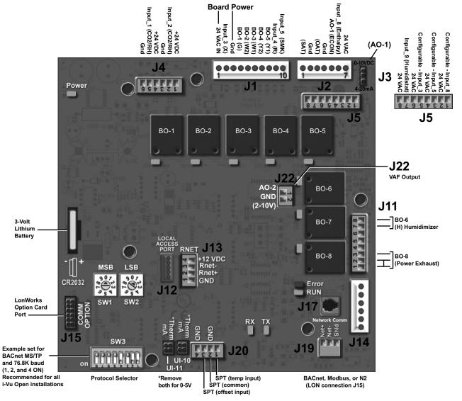
Fig. 51 — RTU Open Control Module
