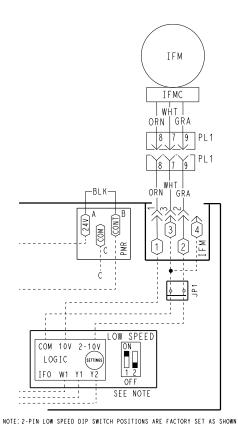
Fig. 10 — Supply Fan Control Wiring Diagram
