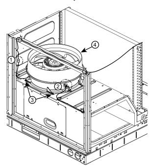
Fig. 11 — Fan Assembly Removal
