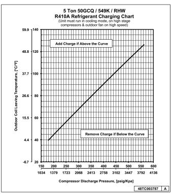
Fig. 24 — Cooling Charging Chart - 5 Ton
