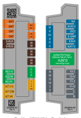
Fig. 68 — W7220 Wiring Terminals
