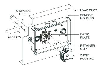
Fig. 48 — Sensor Cleaning Diagram
