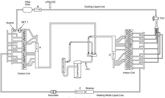
Fig. 19 — Typical Piping Schematic
