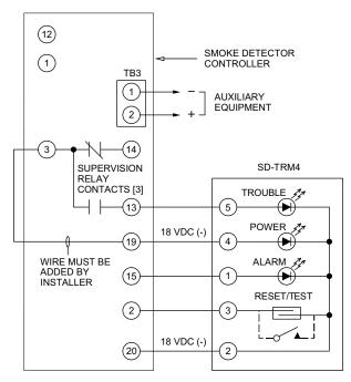
Fig. 47 — Remote Test/Reset Station Connections
