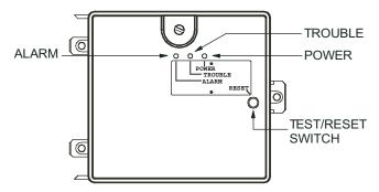
Fig. 49 — Controller Assembly
