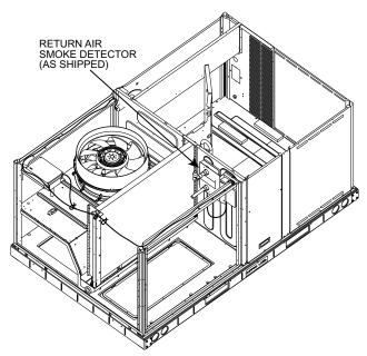
Fig. 42 — Typical Return Air Smoke Detector Location
