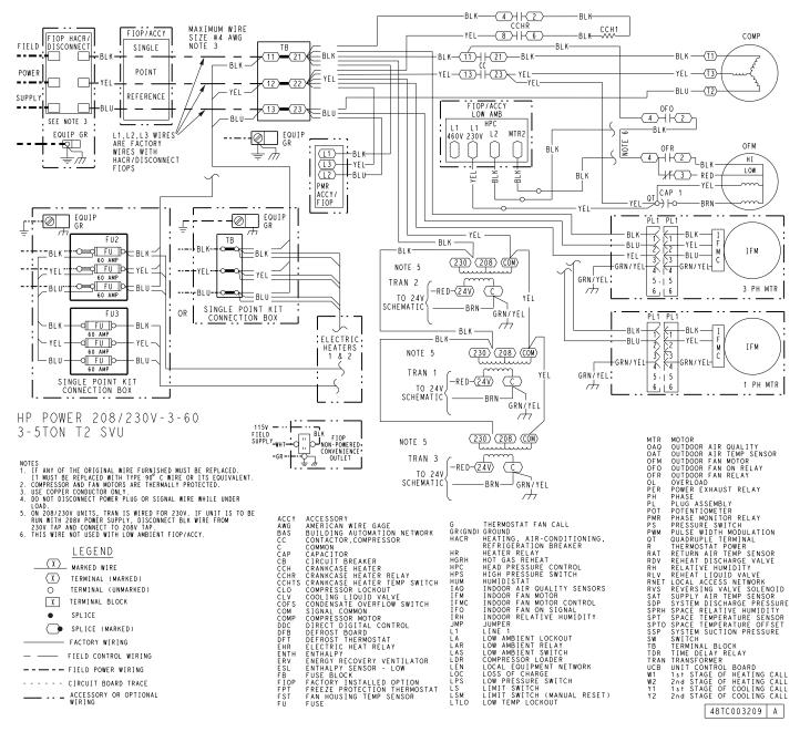
Fig. K — 50GCQ 04-06 SystemVu<sup>™</sup> Power Wiring Diagram — 208/230-3-60
