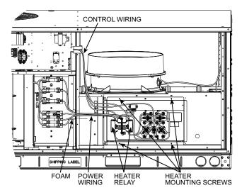
Fig. 36 — Typical Single Point Installation
