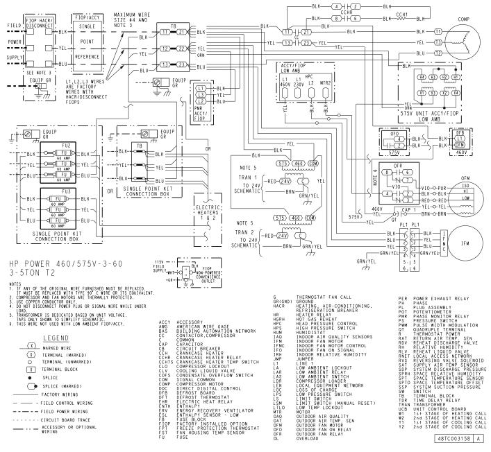
Fig. I — 50GCQ 04-06 Power Wiring Diagram — 460/575-3-60
