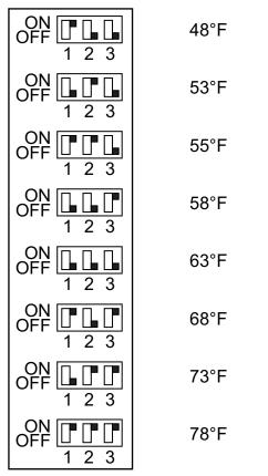
Fig. 60 — Outdoor Air Temperature Changeover Set Points
