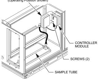
Fig. 45 — Return Air Smoke Detector **Operating Position**
