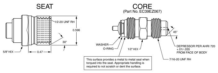
Fig. 21 — CoreMax<sup>1</sup> Access Port Assembly
