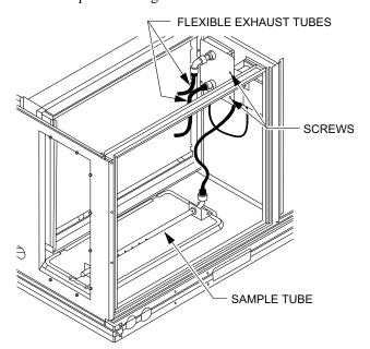
Fig. 44 — Return Air Smoke Detector Shipping Position
