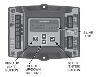
Fig. 71 — W7220 Controller Navigation Buttons
