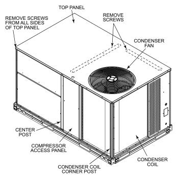
Fig. 15 — Location of Screws and Coil Corner Post
