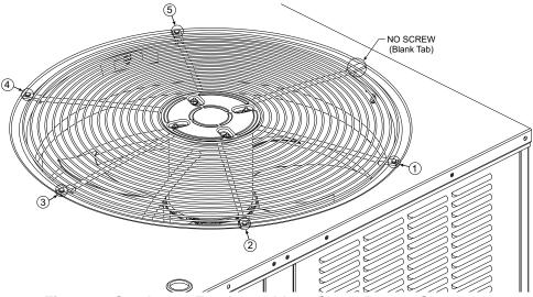
Fig. 26 — Condenser-Fan Assembly — Screw Pattern Sequence
