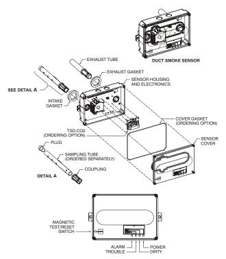
Fig. 40 — Smoke Detector Sensor
