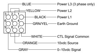
Fig. 6 — ECM Motor Plug Connectors
