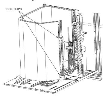
Fig. 17 — Condenser Coil Clips
