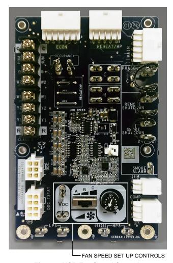
Fig. 7 — UCB Fan Speed Controls
