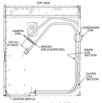
Fig. 18 — Separating Coil Sections
