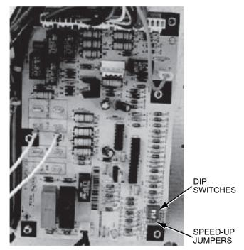
Fig. 30 — Defrost Control Board Arrangement
