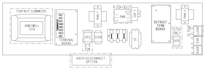
Fig. 31 — Defrost Control Board Location - 50GCQ 04-06 Electro-Mechanical Units
