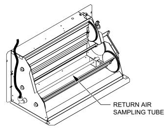
Fig. 43 — Return Air Sampling Tube Location (View reoriented to show opposite side for clarity.)
