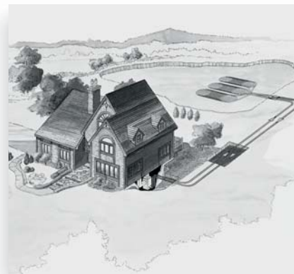
Ground Water (open) Loop
