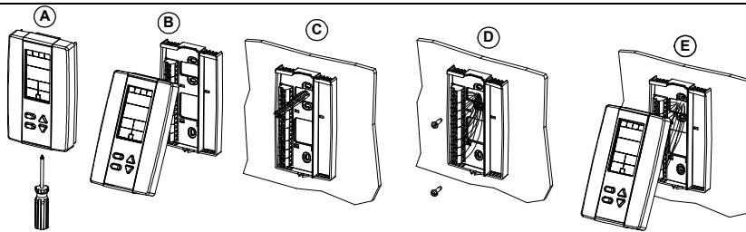
CAUTION: Risk of malfunction. Remove power prior to separate thermostat cover from its base.
