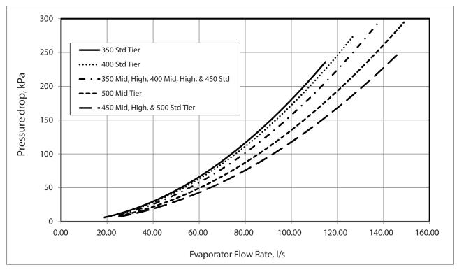
NOTE: The indicated pressure drop is from the inlet to the outlet of the evaporator. This does not consider other system components or whether or not a factory-supplied hydronic kit is employed.
