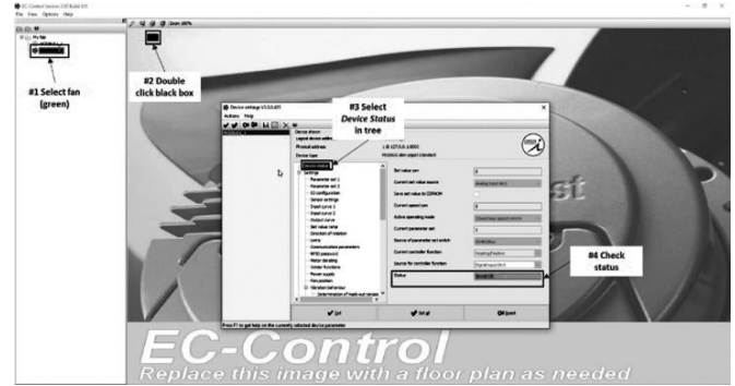
Fig. 21 — EC-Control Fan Connection Verification
