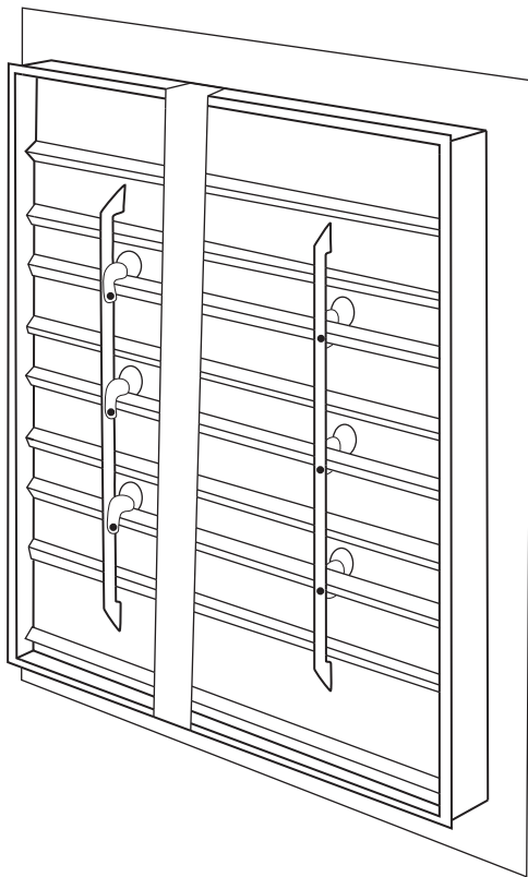
Fig. 14 — Optional Exhaust Damper
