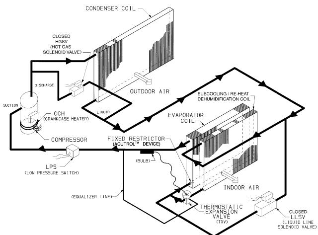
**Fig. 51 — Humidi-MiZer Subcooling Mode Operation**
