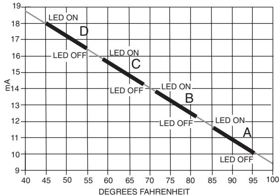
**Fig. 39 — Outdoor Air Temperature Changeover Set Points**
