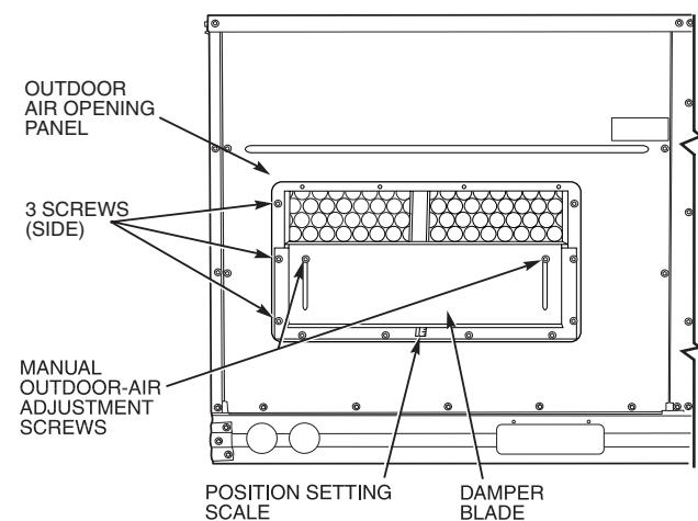
**Fig. 17 — Damper Panel with Manual Outdoor-Air Damper Installed**
