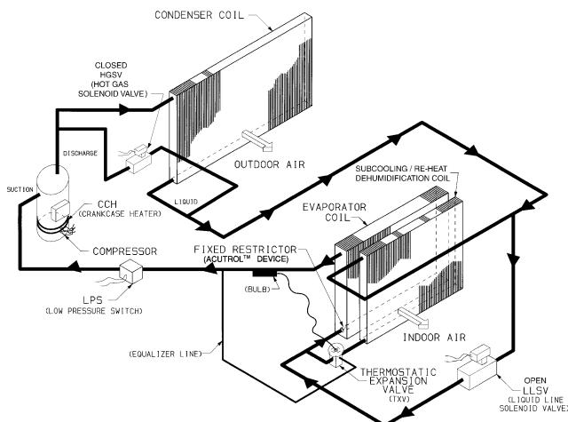
**Fig. 50 — Humidi-MiZer Normal Design Cooling Mode Operation**
