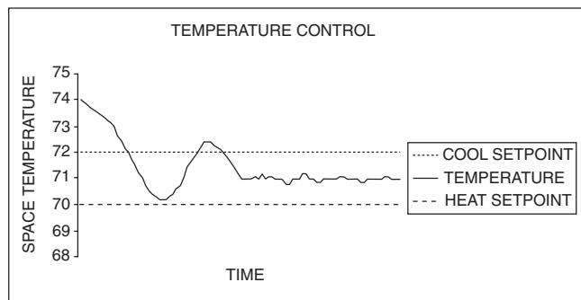
**Fig. 49 — Economizer Temperature Control Example**
