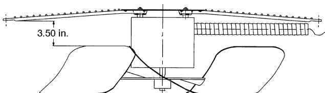
**Fig. 56 — Condenser-Fan Adjustment**
