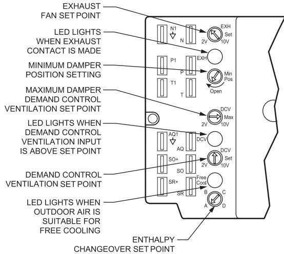
**Fig. 38 — EconoMi\$er IV Controller Potentiometer and LED Locations**
