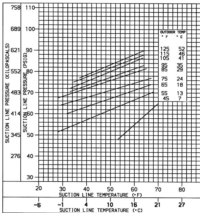
Fig. 58 — Cooling Charging Chart, Standard 48HJ009 Units
