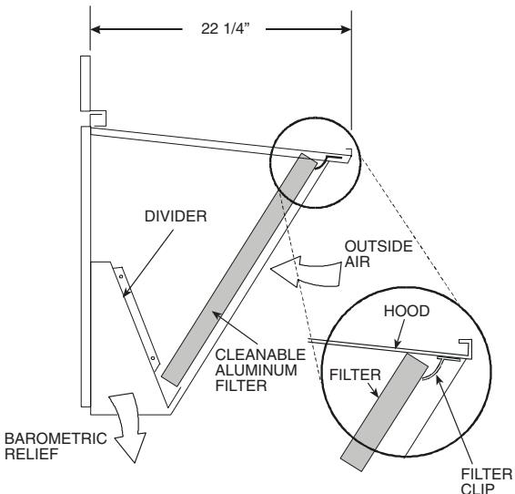
**Fig. 31 — Filter Installation**
