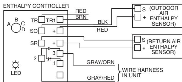
**Fig. 23 — Outdoor and Return Air Sensor Wiring Connections for Differential Enthalpy Control**
