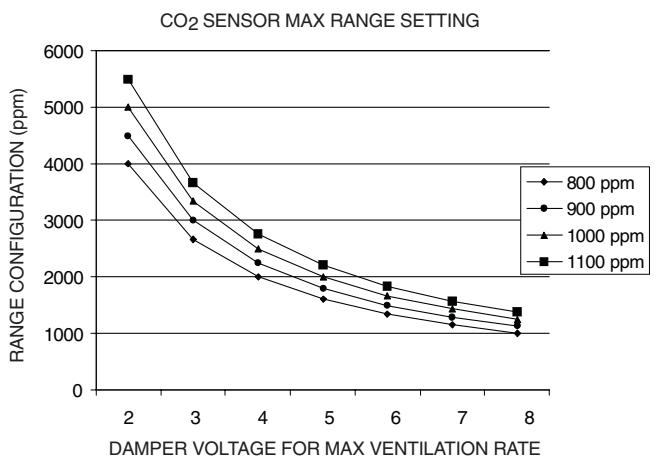
**Fig. 43 — CO<sub>2</sub> Sensor Maximum Range Setting**
