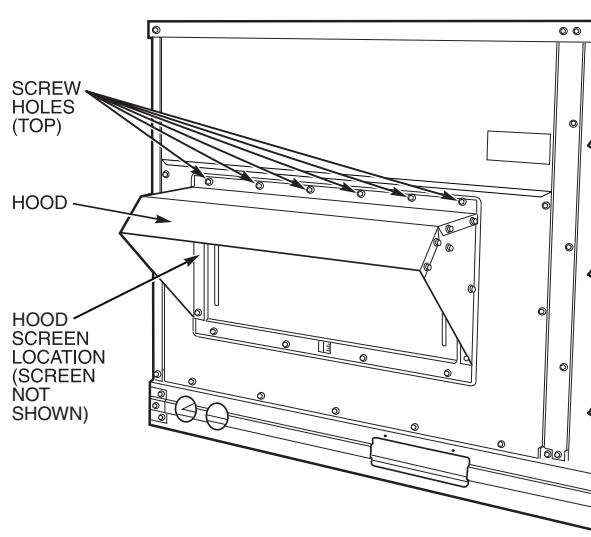
**Fig. 19 — Optional Manual Outdoor-Air Damper with Hood Attached**
