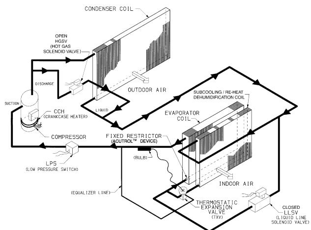
**Fig. 52 — Humidi-MiZer Hot Gas Reheat Mode Operation**
