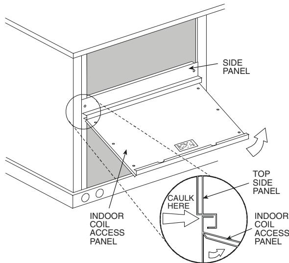
**Fig. 29 — Indoor Coil Access Panel Relocation**
