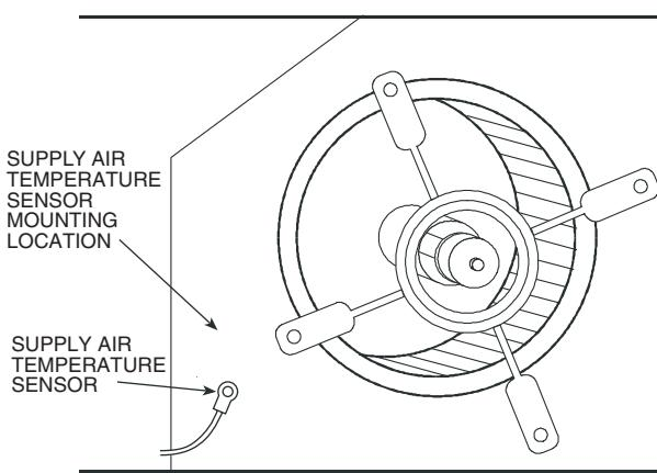
**Fig. 37 — Supply Air Sensor Location**
