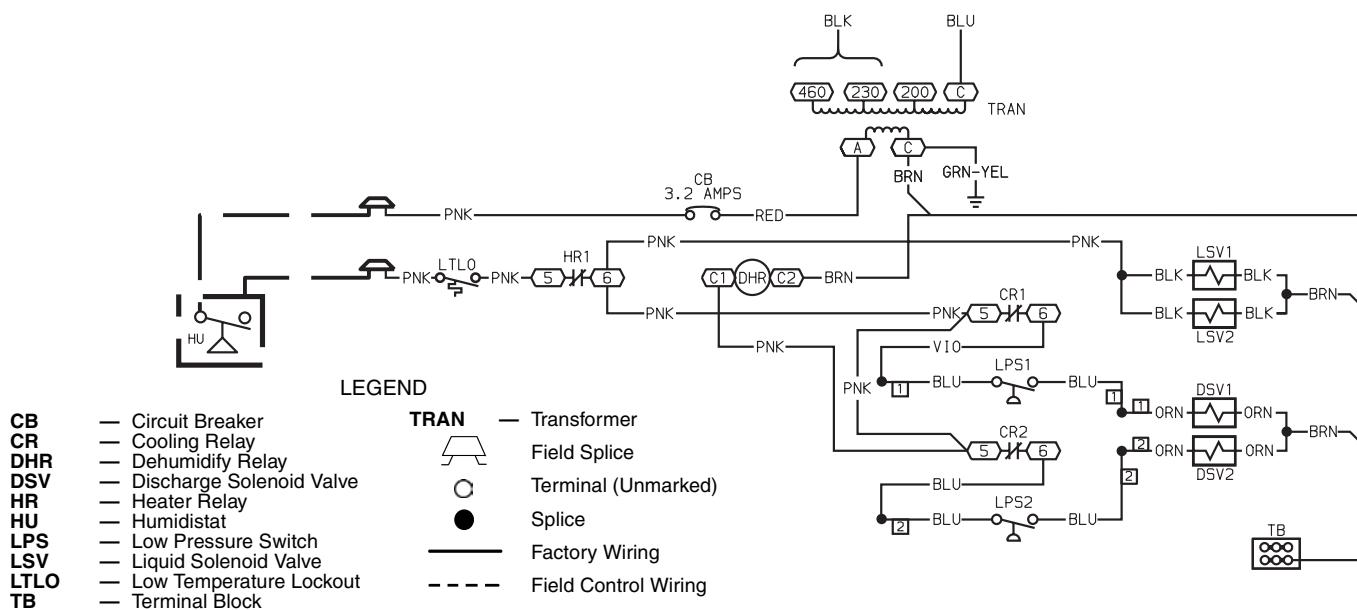
NOTE: The Humidi-Mizer circuit is active when both LLSV1 and LLSV2 are energized.
