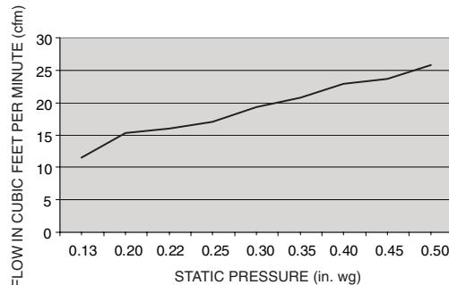
**Fig. 35 — Outdoor Air Damper Leakage**
