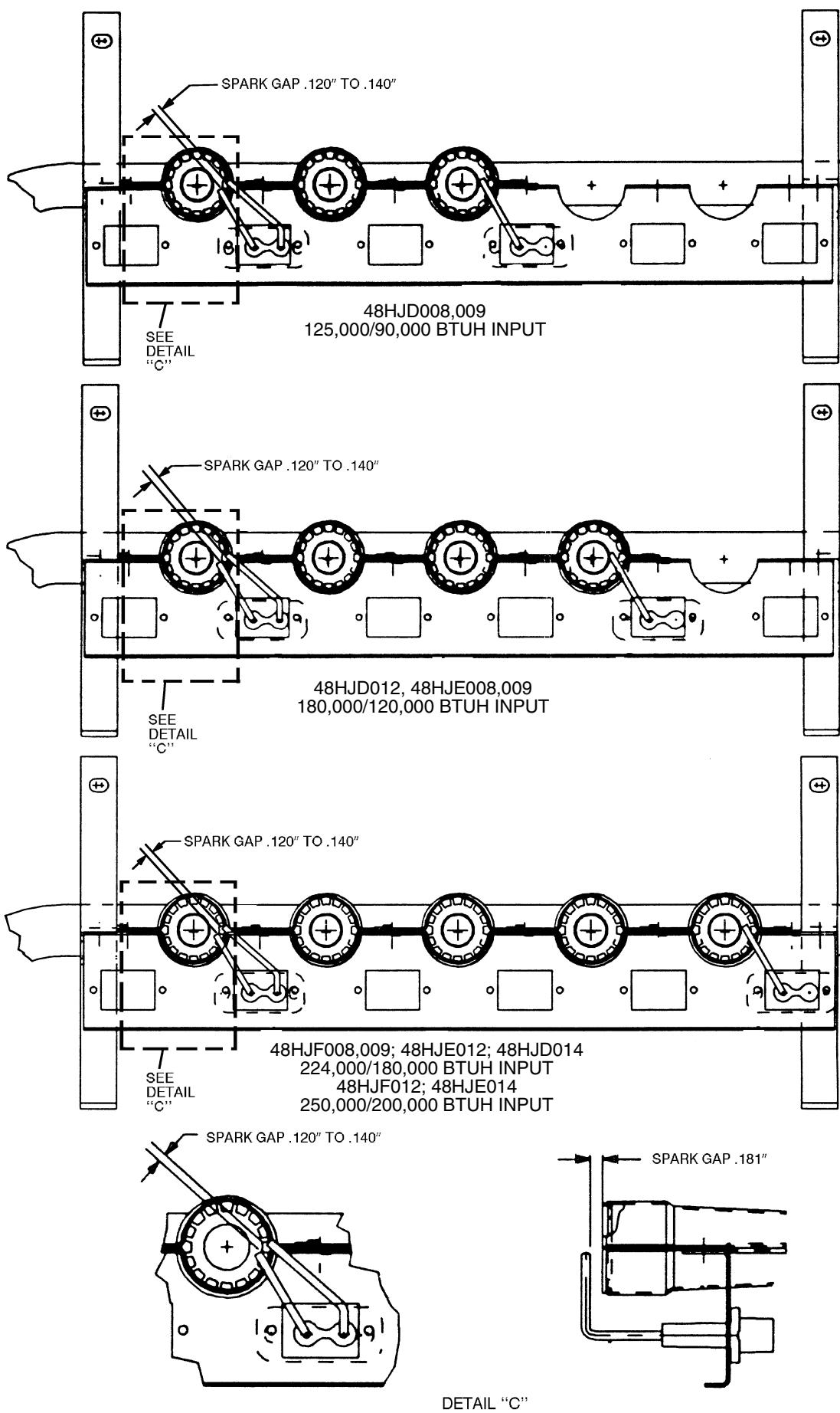
**Fig. 66 — Spark Gap Adjustment**
