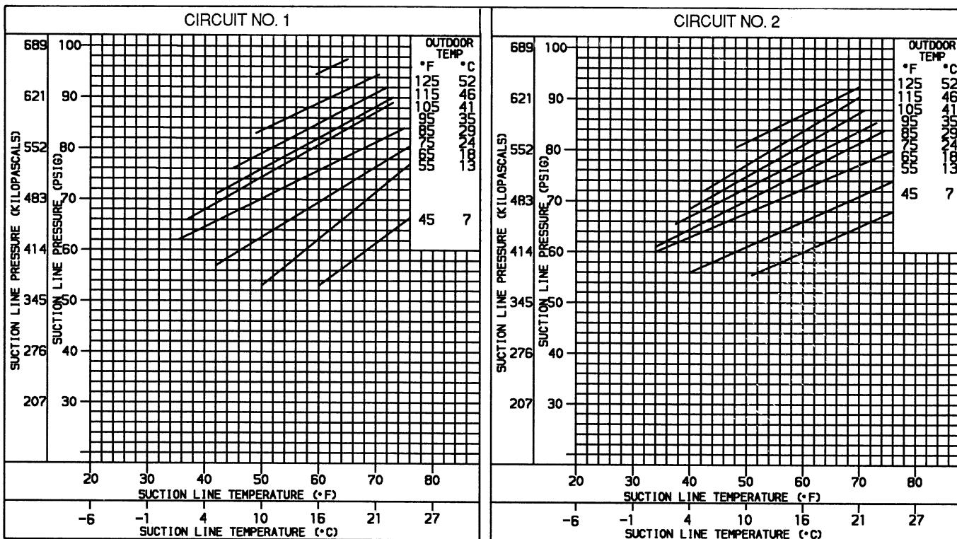
Fig. 60 — Cooling Charging Charts, Standard 48HJ014 Units
