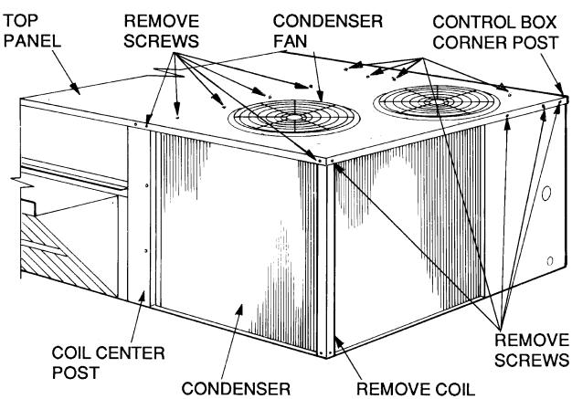
**Fig. 53 — Cleaning Condenser Coil**
