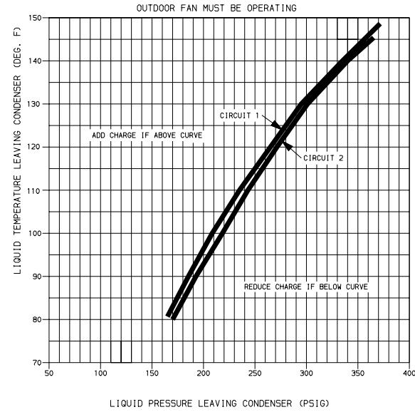
NOTE: When using the charging charts, it is important that only the subcooling/reheat dehumidification coil liquid line solenoid valve be energized. The subcooling/reheat dehumidification coil liquid line solenoid valve MUST be energized to use the charging charts and the outdoor motor speed controller jumpered to run the fan at full speed.
