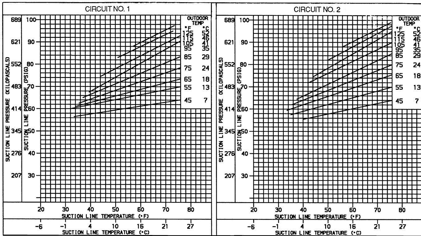
Fig. 59 — Cooling Charging Charts, Standard 48HJ012 Units
