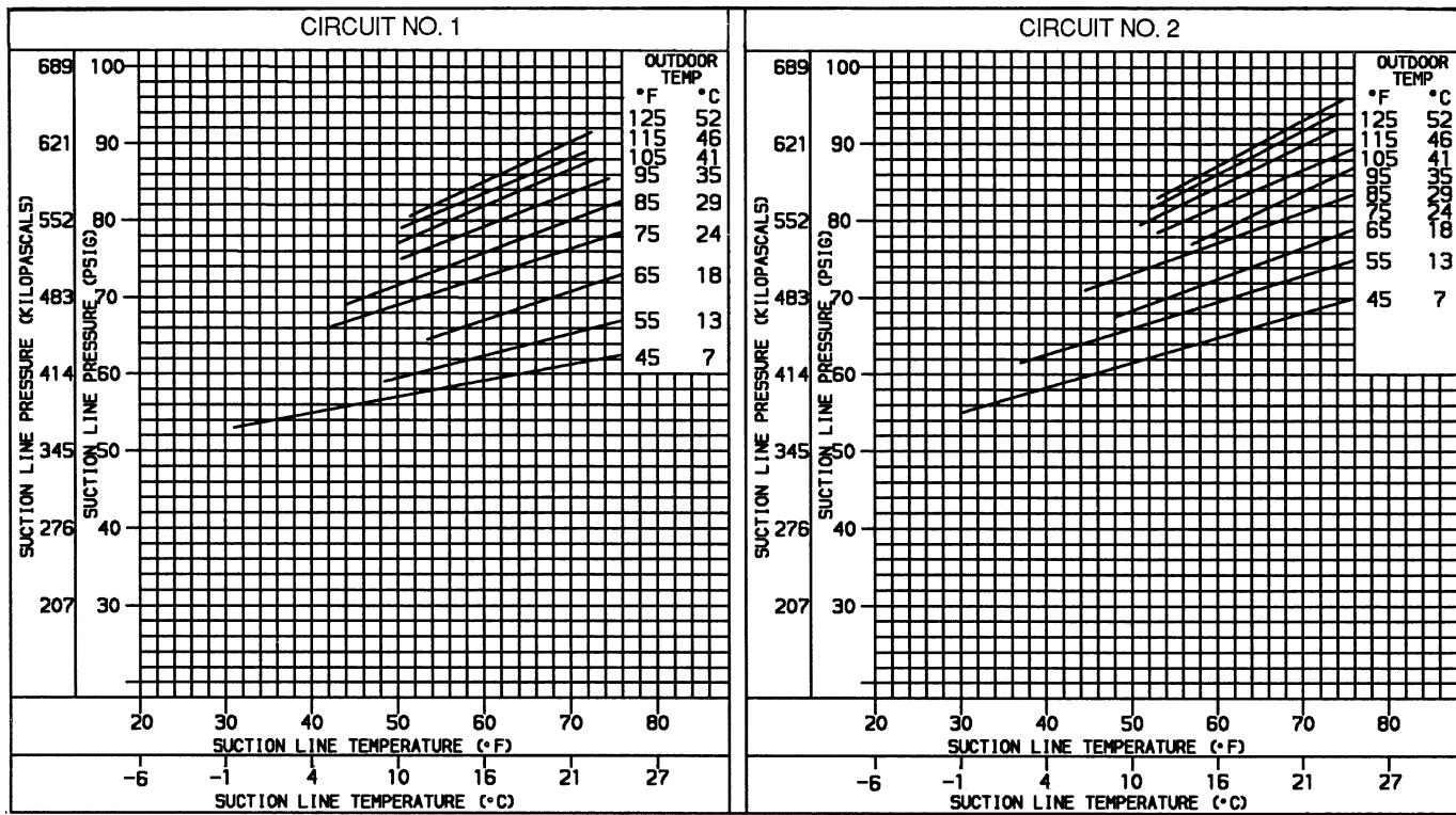
Fig. 57 — Cooling Charging Charts, Standard 48HJ008 Units
