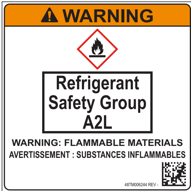
Fig. 60 — A2L Refrigerant Safety Group Warning Label
