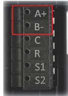
Fig. 11 — BACnet Communication Wiring
