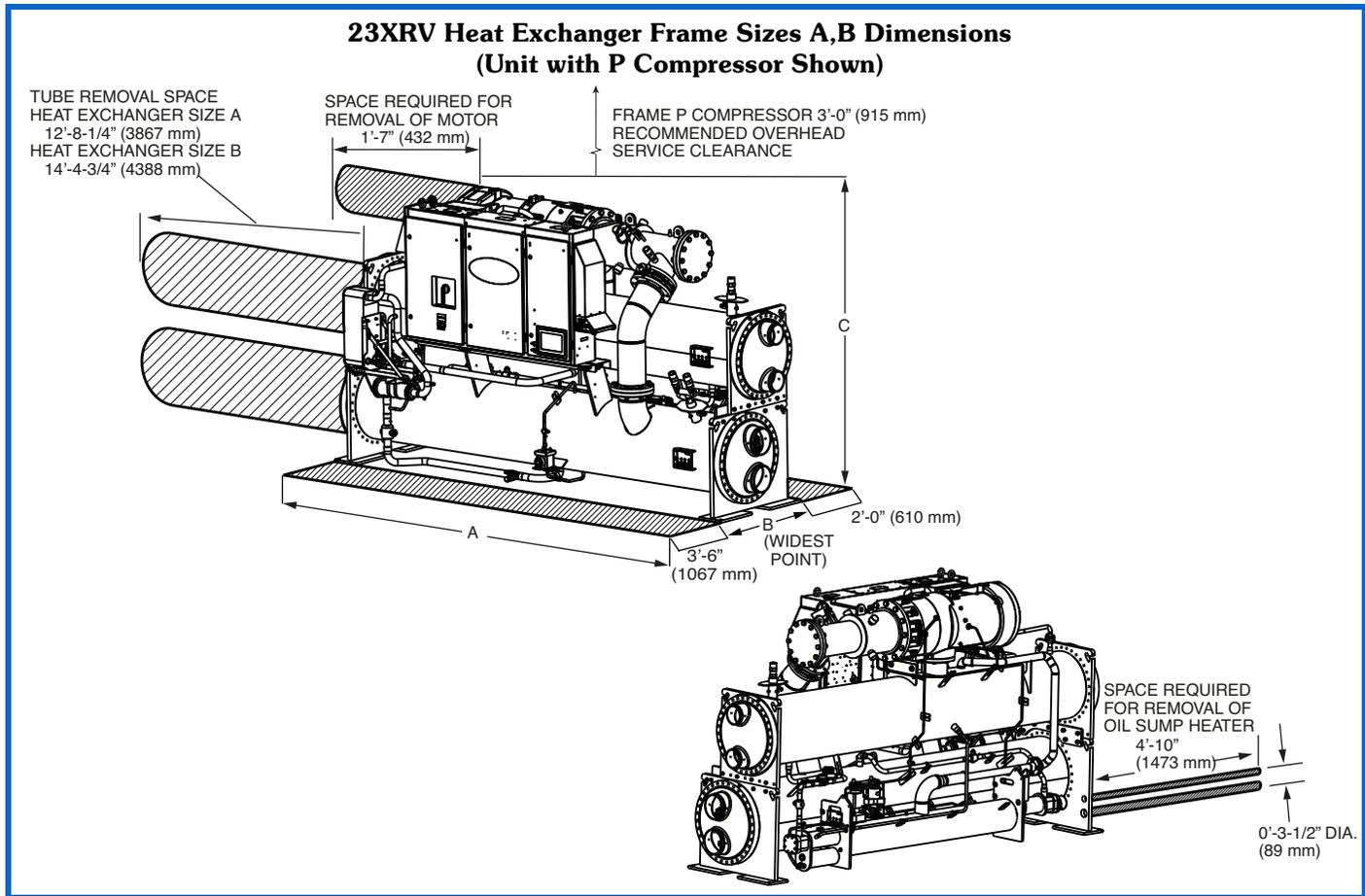
**23XRV Heat Exchanger Sizes A,B Dimensions (Nozzle-in-Head Waterbox)<sup>a,b,c,d,e,f</sup>**
