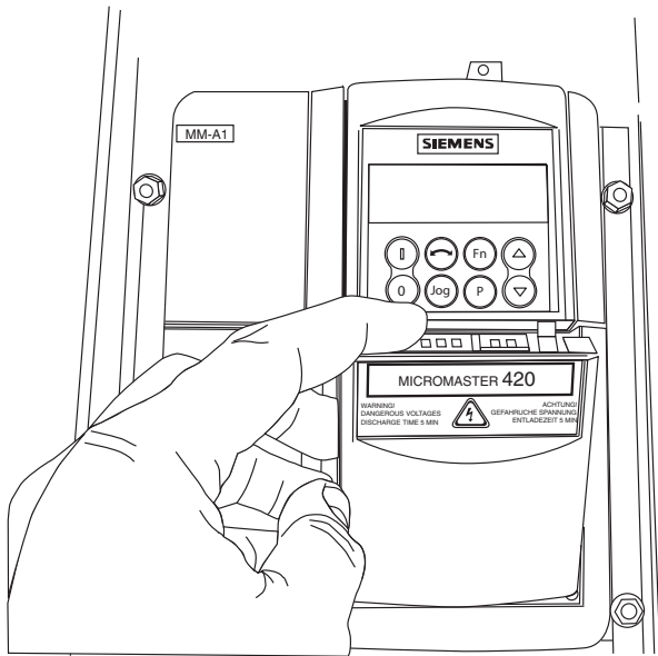
Fig. 21 — Removing Lower Cover (Siemens)
