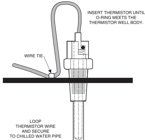
**Fig. 60 — Dual Chiller Accessory Kit Leaving Water Thermistor and Well (Part No. 00EFN900044000A)**
