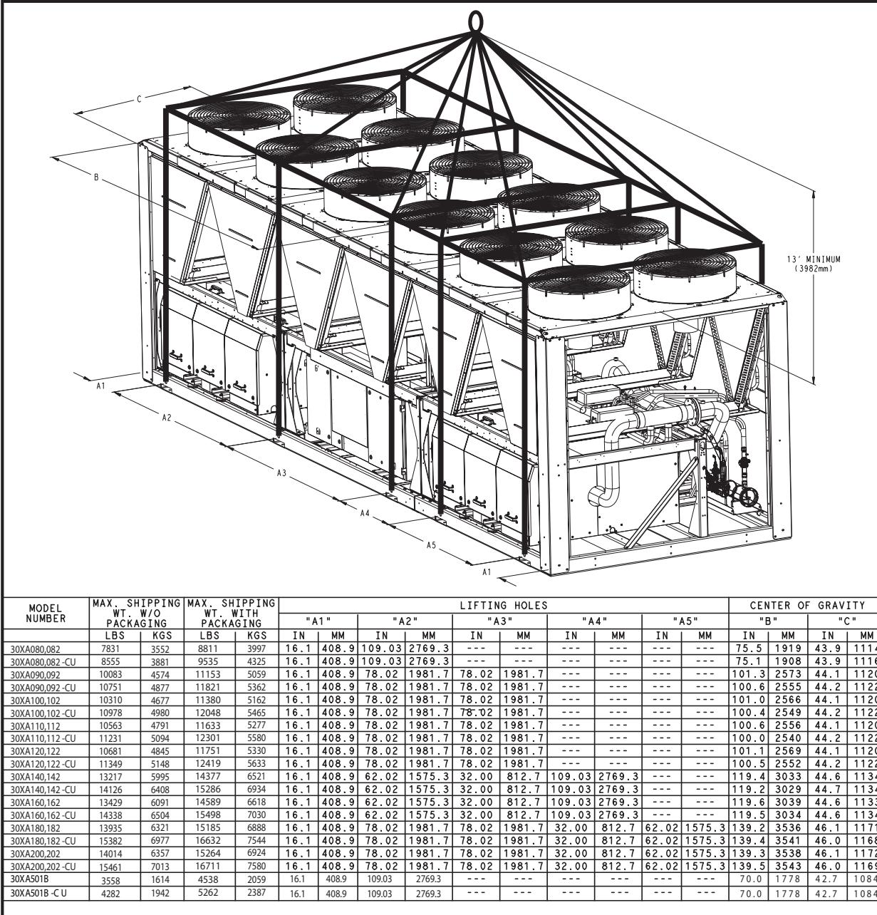
**Fig. 29 — Unit Rigging Label Detail 30XA080-202, 501B**
