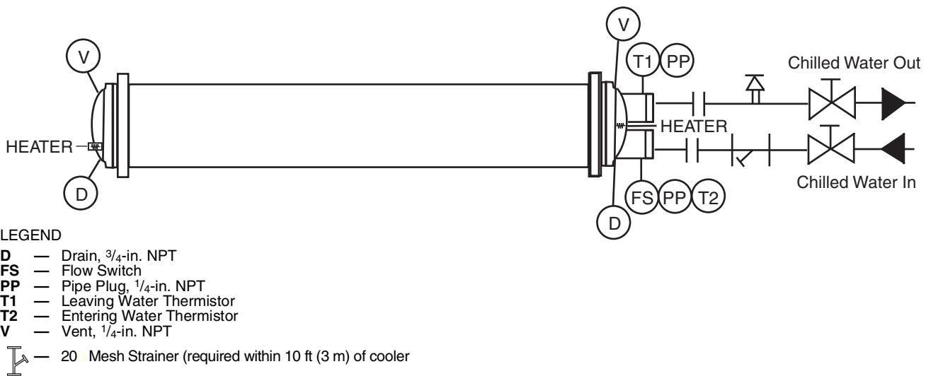
**Fig. 45 — Typical Piping Diagram on 30XA Units without Hydronic Package (Flooded Cooler)**
