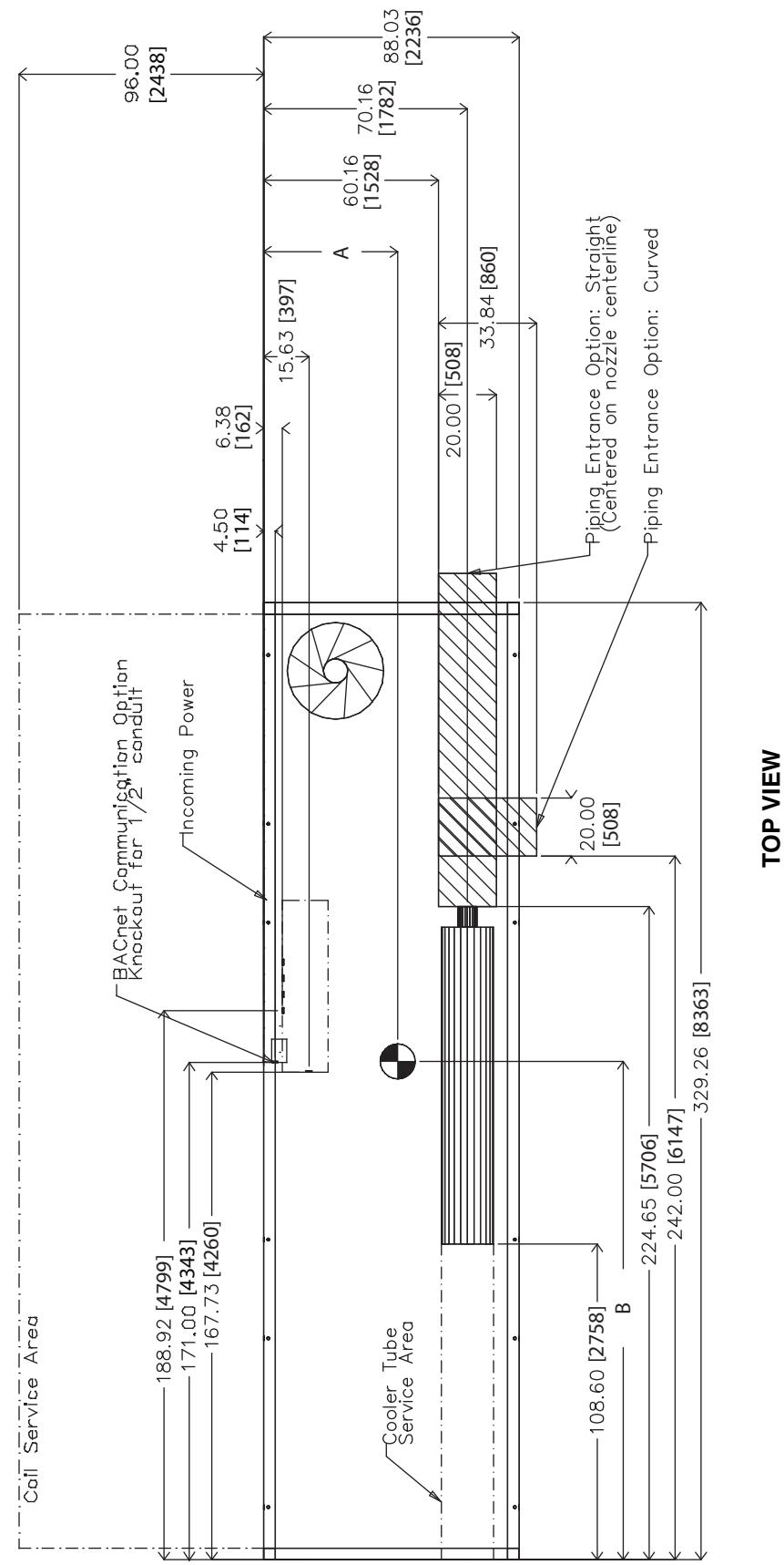
**Fig. 13 — 30XA220/240 Air-Cooled Liquid Chiller Dimensions (See Note 4)**
