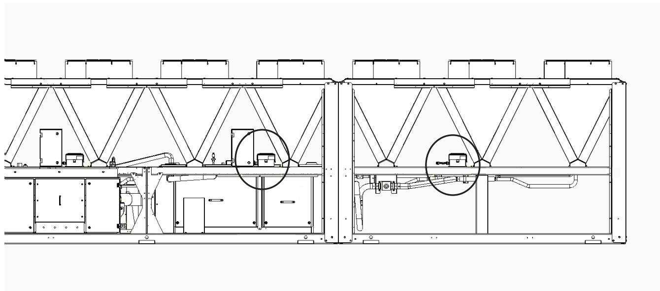
**Fig. 34 — 30XA501 Fan Junction Boxes to be Connected with Conduit Jumper**
