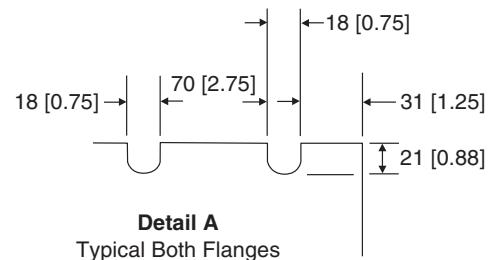
**Fig. 53 — Field-Fabricated and Field-Installed Wind Baffles**
