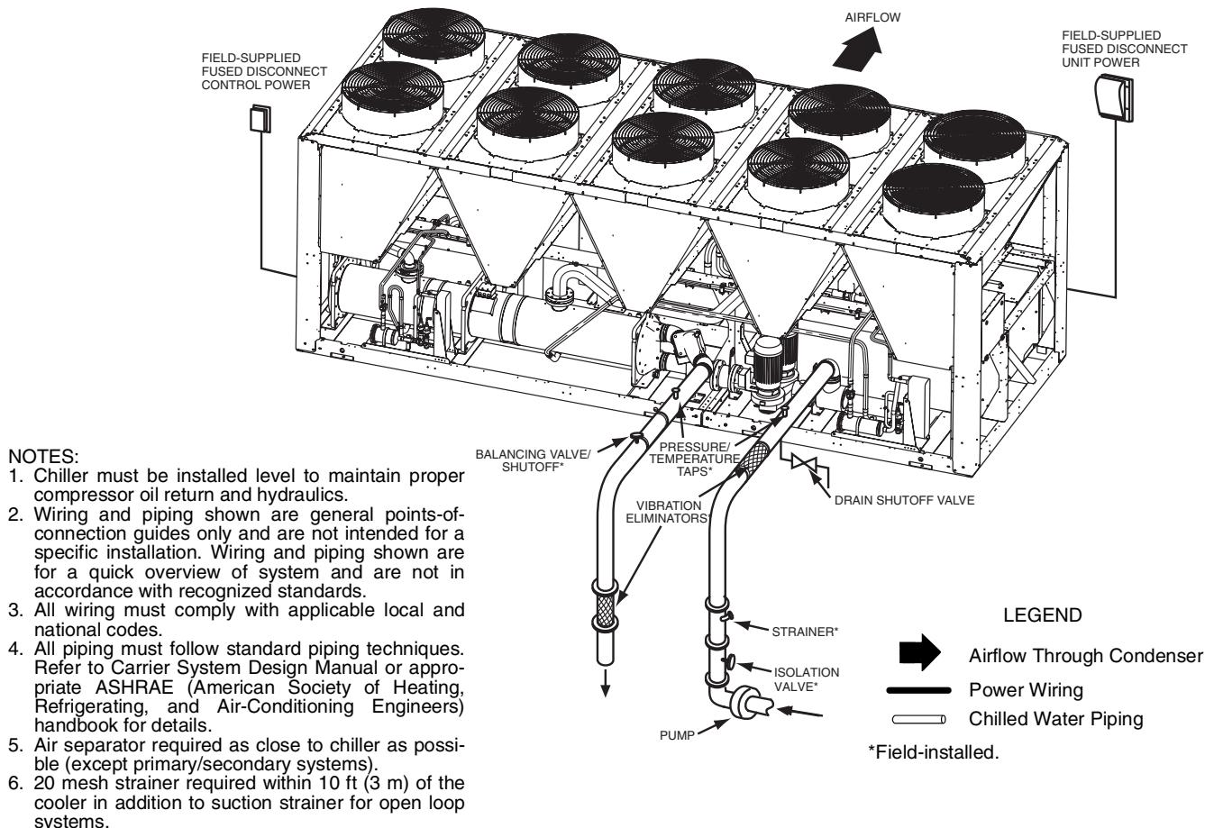
**Fig. 37B — 30XA Flooded Cooler Typical Piping and Wiring (Units with Hydronic Package)**
