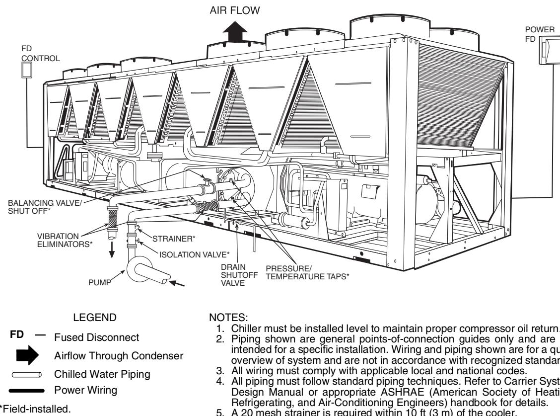
**Fig. 37A — 30XA Flooded Cooler Typical Piping and Wiring (Units without Hydronic Package)**
