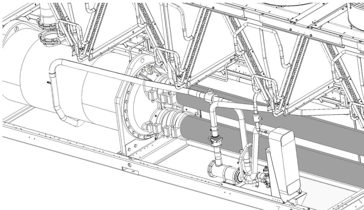
**Fig. 36 — 30XA476, 501 Water Line Connection Using 2 No. 13 Victaulic Elbows Per Line from the Side of the Unit**
