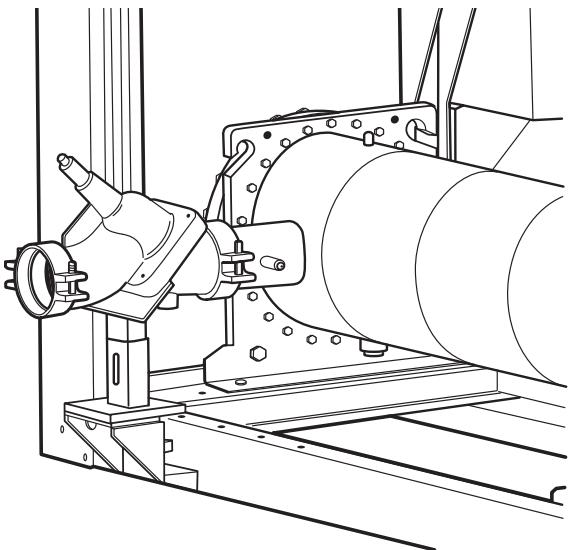
**Fig. 52 — Balancing Valve**
