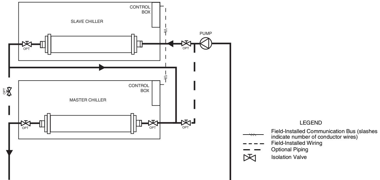
**Fig. 47 — Series Dual Chiller Operation (Not Recommended for DX Cooler)**
