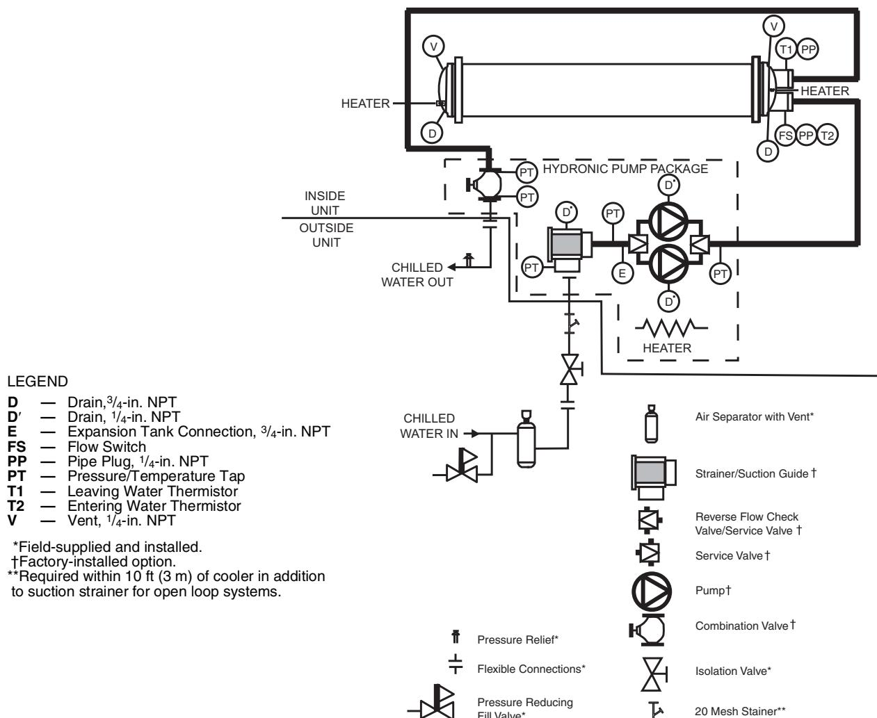
**Fig. 43 — Typical Piping Diagram on 30XA Units with Hydronic Package — Dual Pumps (Flooded Cooler)**
