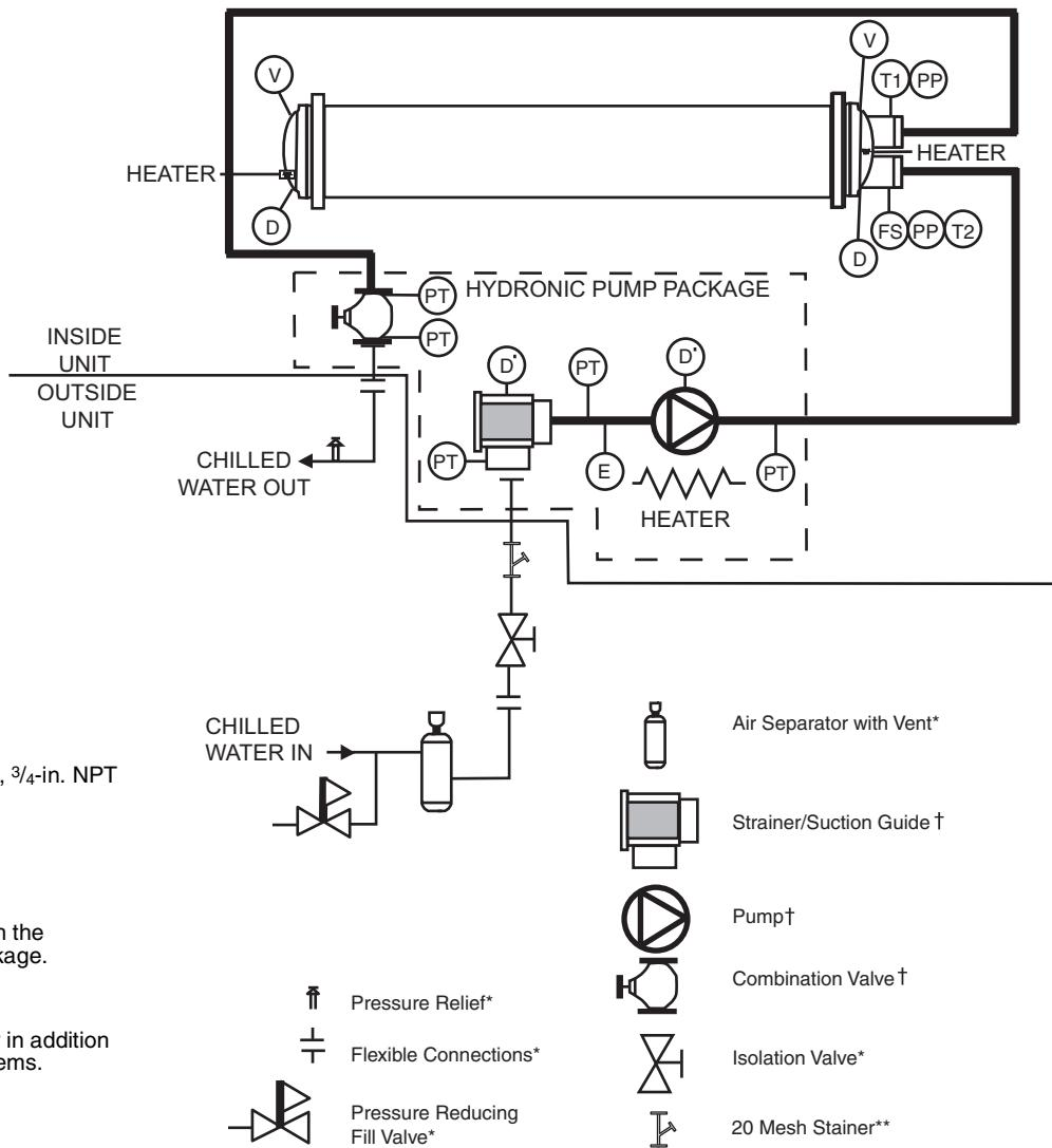
**Fig. 42 — Typical Piping Diagram on 30XA Units with Hydronic Package — Single Pump (Flooded Cooler)**
