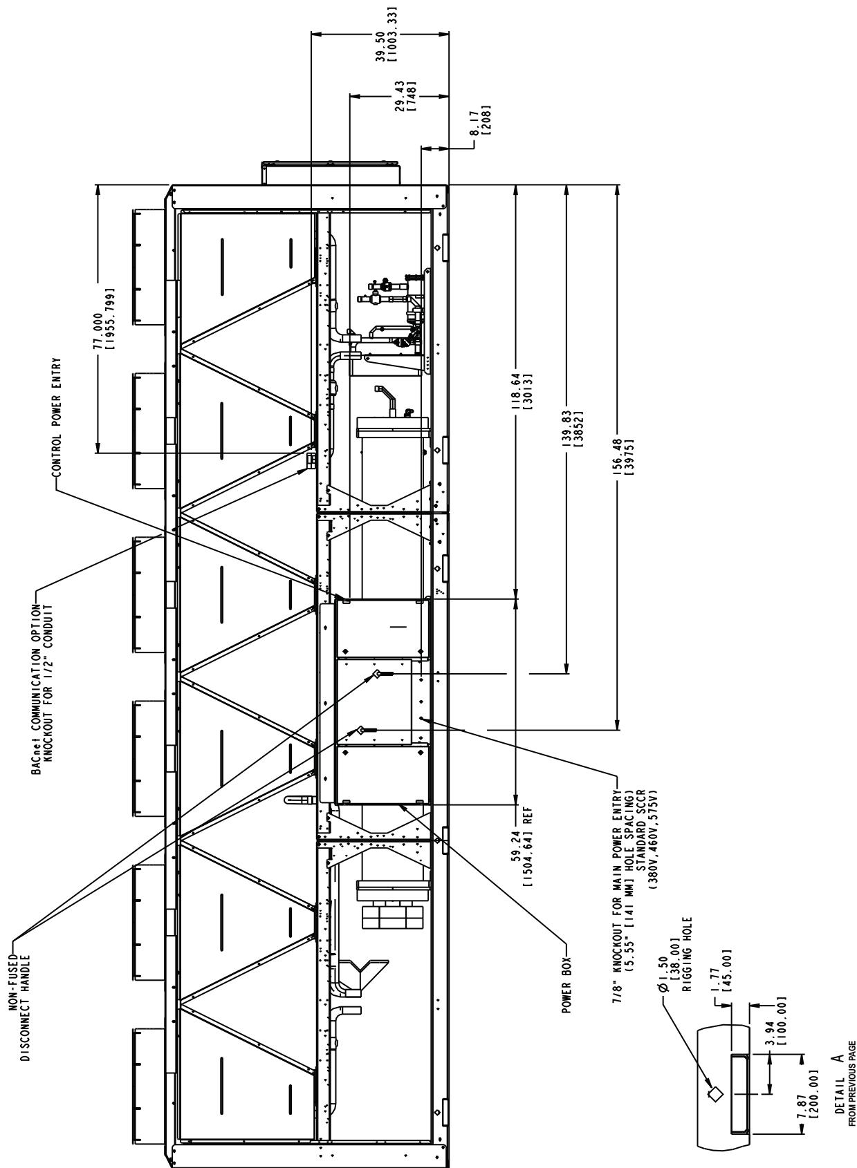
Fig. 12 — 30XA182,202 Air-Cooled Liquid Chiller Dimensions (cont)
