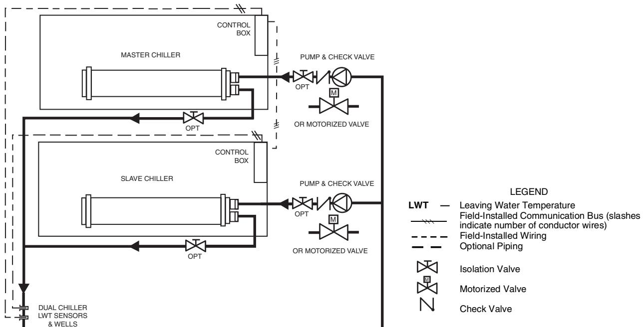
**Fig. 46 — Parallel Dual Chiller Operation**
