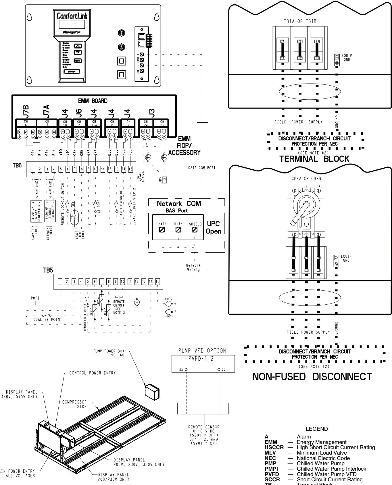
Fig. 58 — Control and Power Wiring Schematic
