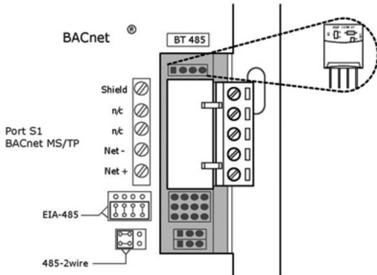
**Fig. 63 — BT485 Terminator Installation**
