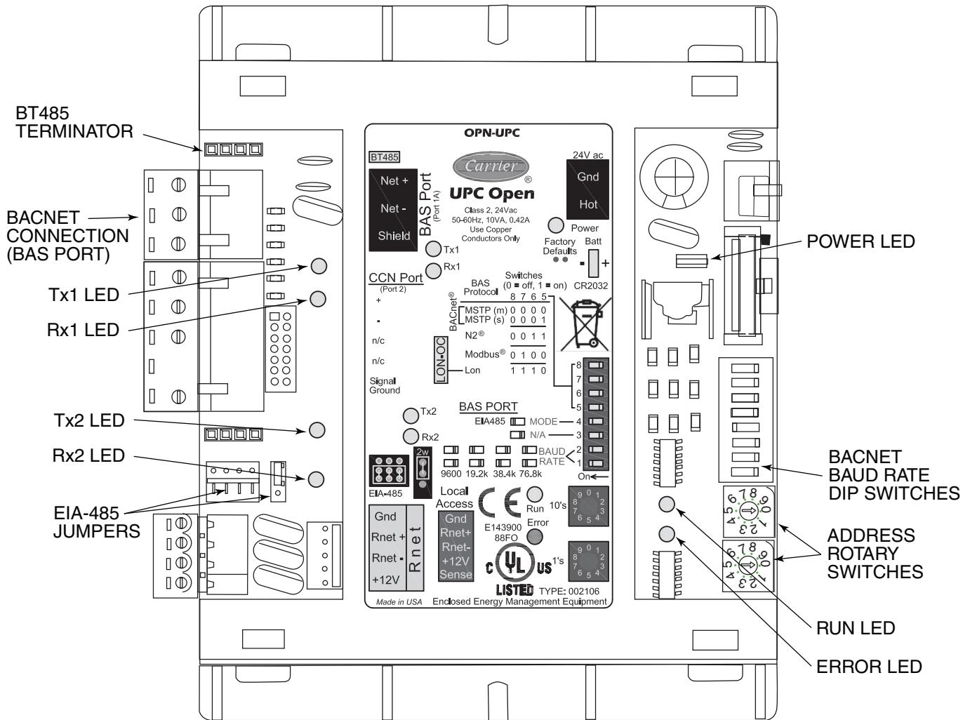
Fig. 61 — UPC Open Controller
