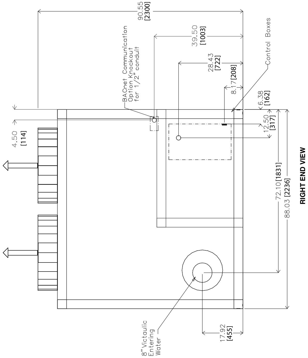
**Fig. 20 — 30XA400 Single Point Air-Cooled Liquid Chiller Dimensions (cont)**
