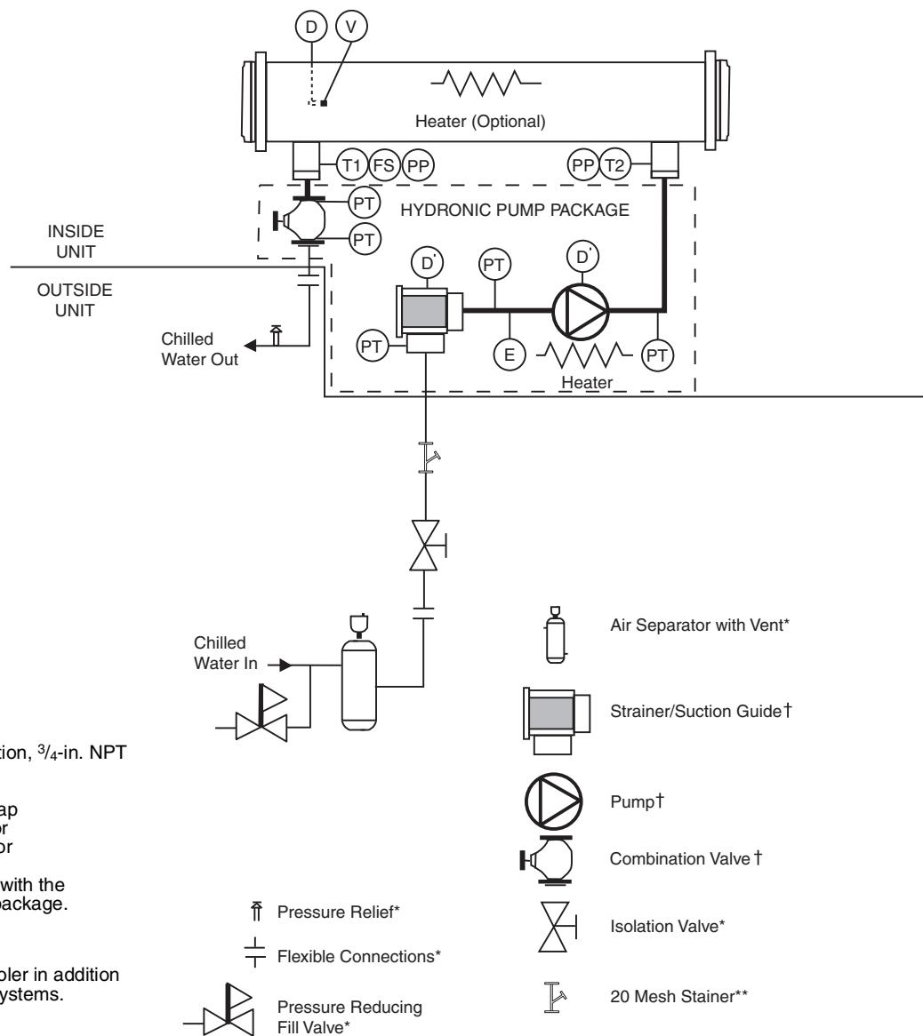
**Fig. 49 — Typical Piping Diagram on 30XA DX Cooler Units with Hydronic Package — Single Pump**
