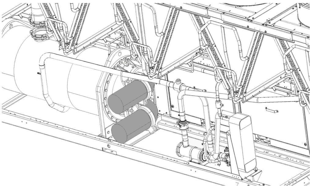
**Fig. 35 — 30XA401, 451, 476, 501 Water Line Installation Using Elbows**
