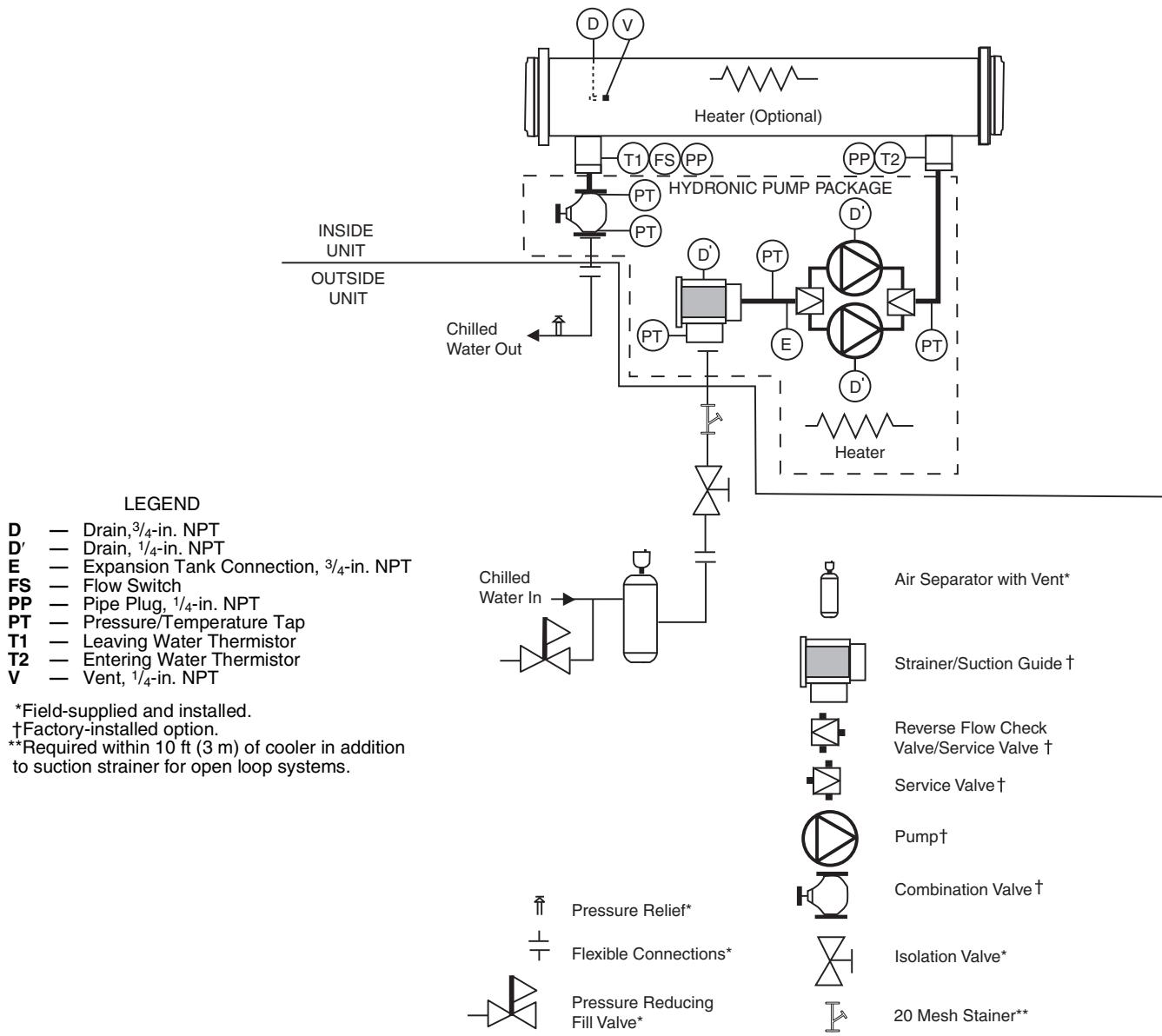
Fig. 50 — Typical Piping Diagram on 30XA DX Cooler Units with Hydronic Package — Dual Pumps
