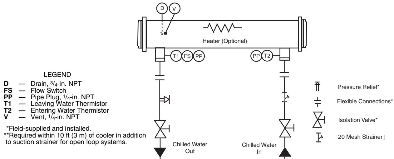
Fig. 51 — Typical Piping Diagram on 30XA082, 092, 102, 112, 122, 142, 162, 182, 202 without Hydronic Package
