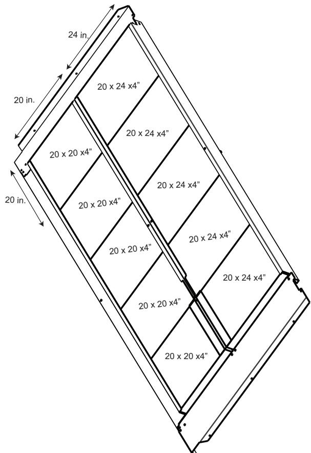
**Fig. 10 — 4 in. Filter Orientation**
