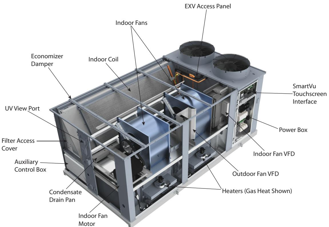
**Fig. 3 — 50K Key Component Locations (48K Size 20-34 Shown)**
