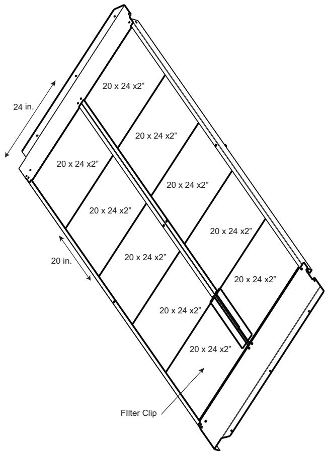
**Fig. 9 — Filter Clip and 2 in. Filter Orientation**
