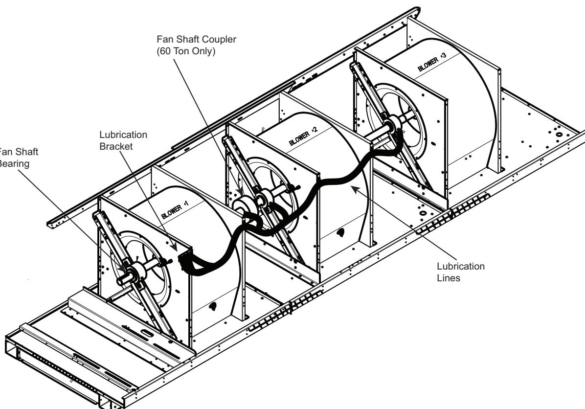
**Fig. 13 — 60 Ton Fan Shaft with Extended Lubrication Lines**
