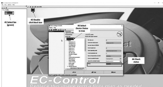
Fig. 15 — EC-Control Fan Connection Verification
