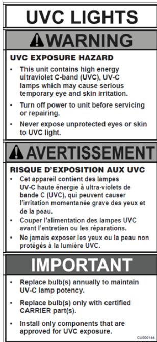
Fig. 13 — UV-C Light Warning Labels Factory Placed on External Side of Cooling Coil Section Access Panels
