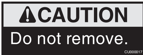
Fig. 4 — Panel Removal Warning Sticker — Factory Placed on External Side of Cooling Coil Section Top Panel
