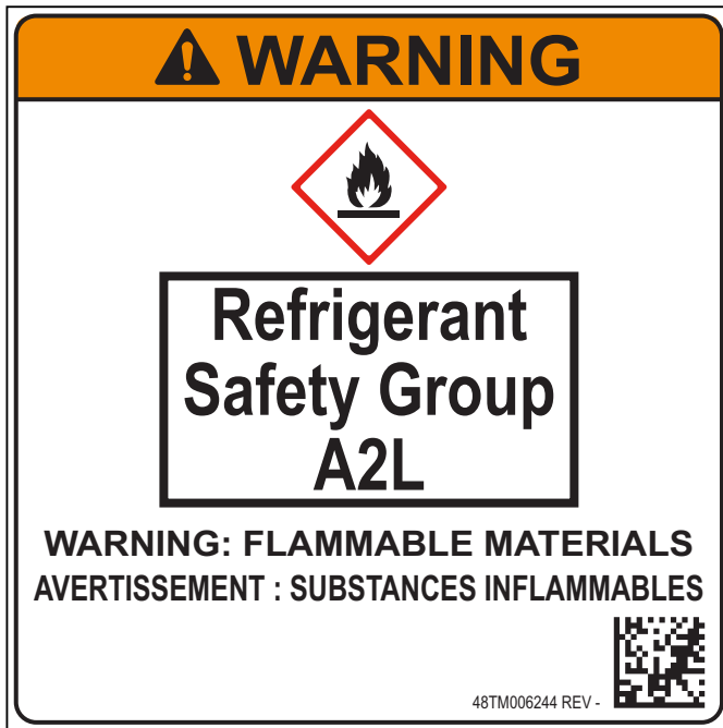
Fig. 57 — A2L Refrigerant Safety Group Warning Label
