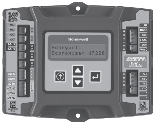
The W7220 economizer module can be used as a stand-alone economizer module wired directly to a commercial set-back space thermostat and sensors to provide outside air dry-bulb economizer control.
