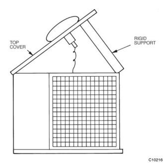
Fig. 34 - Pivot and Support Top Cover
