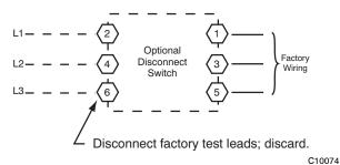
Fig. 11 - Power Wiring Connections
