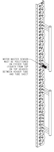
Fig. 38 - 38AUZ\*12 Motormaster Sensor Location (RTPF)
