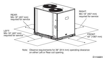
Fig. 4 - Service Clearance Dimensional Drawing
