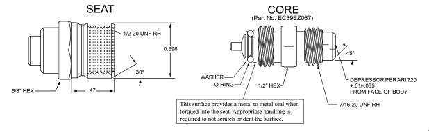
Fig. 26 - CoreMax Access Port Assembly
