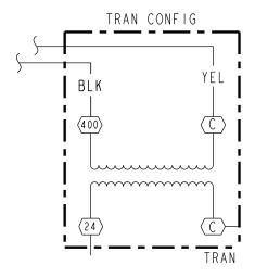
Fig. 14 - Control Transformer Wiring
