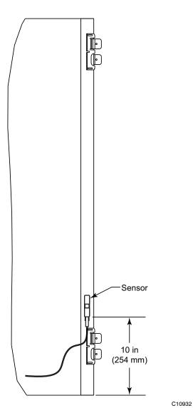
Fig. 36 - 38AUD\*12-14 Motormaster Sensor Location (Novation)
