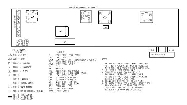
Fig. 24 - Typical 38AUZ Wiring Diagram
