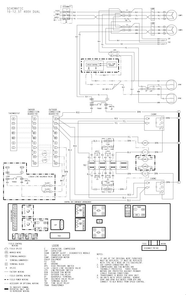
Fig. 25 - Typical 38AUD Wiring Diagram
