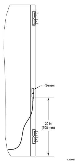
Fig. 35 - 38AUZ Motormaster Sensor Location (All Sizes - Novation)
