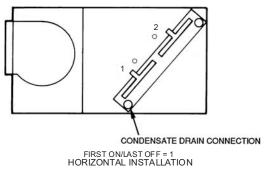
Fig. 6 - Typical Evaporator Coil Connections (40RU)
