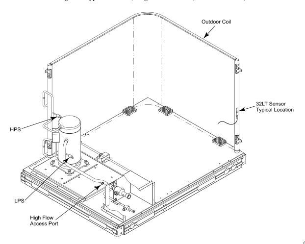
Fig. 30 - Typical Interior, Single-Circuit Unit (38AUZ\*08 shown)
