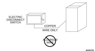
Fig. 10 - Disconnect Switch and Unit
