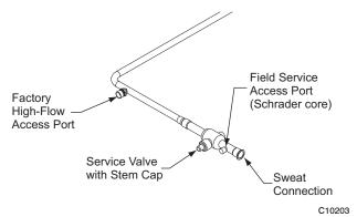
Fig. 9 - Typical Piping Connection Assembly
