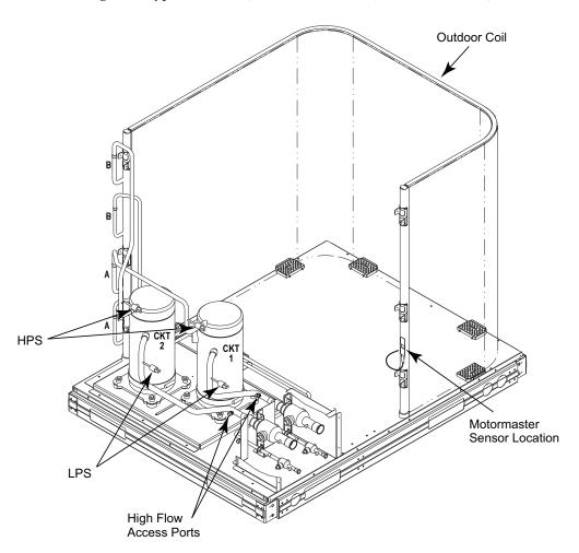
Fig. 32 - Typical Interior, Two-Circuit Unit (38AUD\*14 shown)
