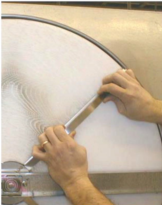
Fig. 29 — Retainer Strap Removal
