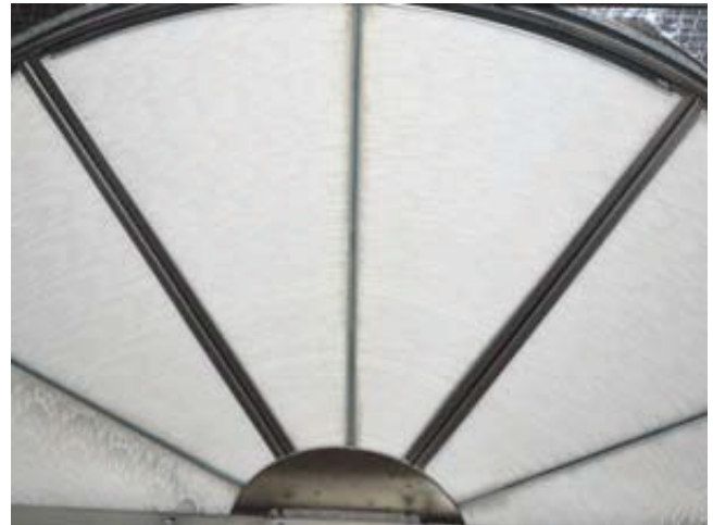
Fig. 31 — Embedded Stiffener Facing Motor Side
