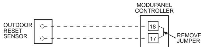
Fig. 18 — Outdoor Reset Sensor Connections
