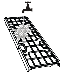
Fig. 18 — Rinse the Filter
