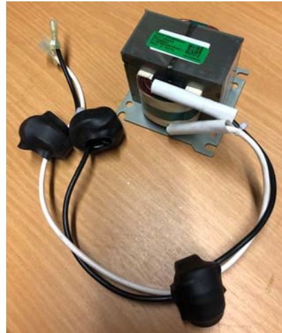
Fig. 28 – 5T Reactor (Note: 5T uses 2 reactors)
