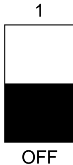
Fig. 47—Example of Setup Switch in OFF Position
