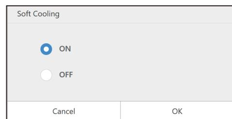
Middle COOL can be turned ON/OFF. When turned ON, the air direction is set to up, and the maximum power is restricted.
