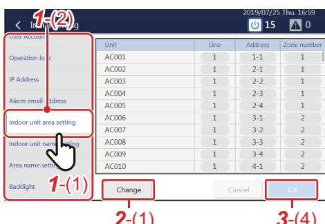
The procedure below is used as an example to explain how to move the indoor unit (AC001) set in area 1 to area 2.
