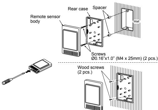
1. Inserting a straight blade screwdriver, etc. into the groove at the lower side of the remote sensor body, force open the rear case to remove it.
