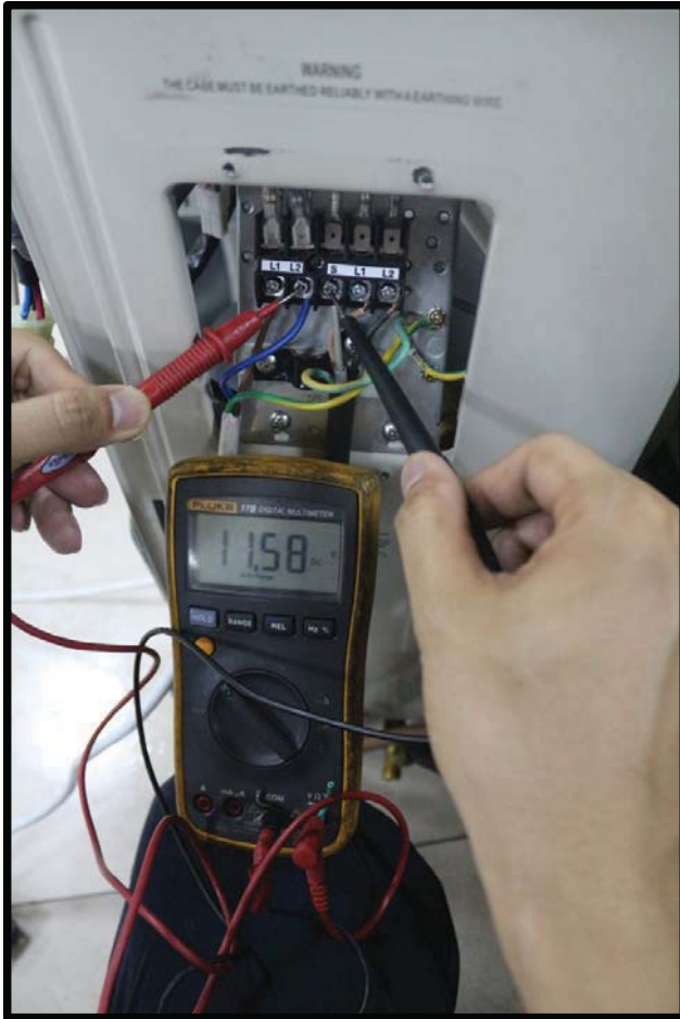
Fig. 30 – Test the DC voltage
