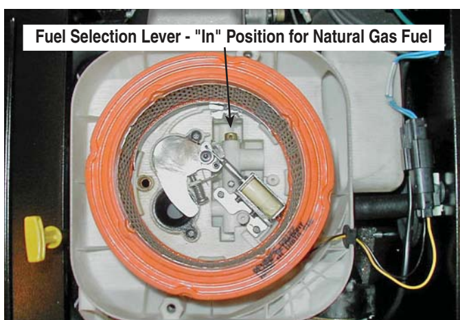
Figure 1.8 - 12, 14, 16, 17, & 20kW, GT-990/GT-999 (Airbox Cover Removed)
