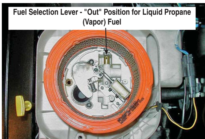
Figure 1.8 - 12, 14, 16, 17, & 20kW, GT-990/GT-999 (Airbox Cover Removed)
