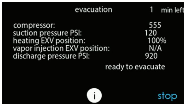
Fig. 25 – Evacuation Status Screen
