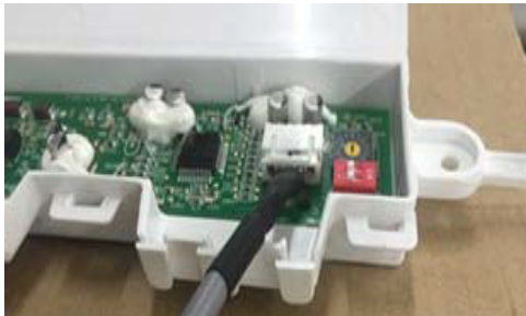
Fig. 24 — Adapter Board to Display Board Connection
