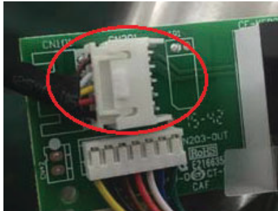
Fig. 19 — CN101 Connection to the Adapter Board
