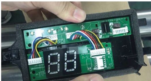
Fig. 22 — Display Board Installed on the Display Board Holder
