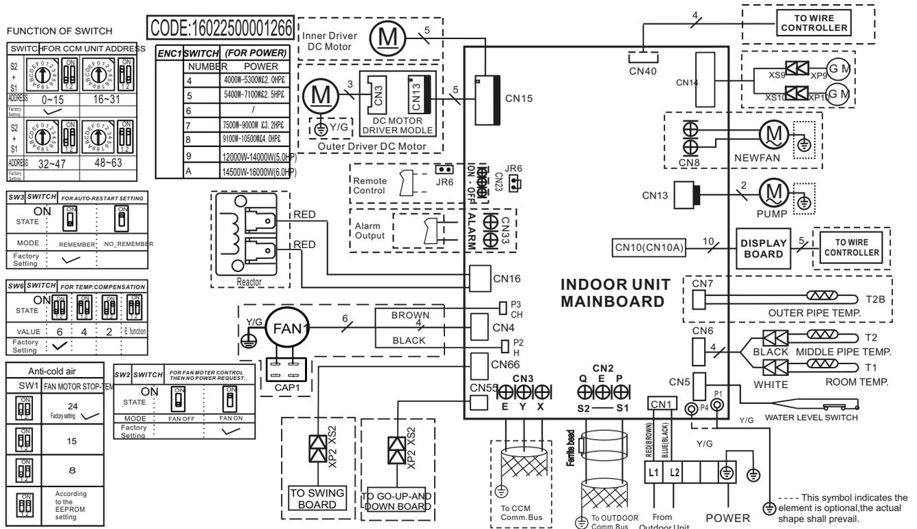
Fig. 7 – Wiring Diagram (Size 36K-48K)
