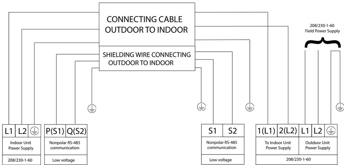
Fig. 4 – Connection Diagrams 36–48
