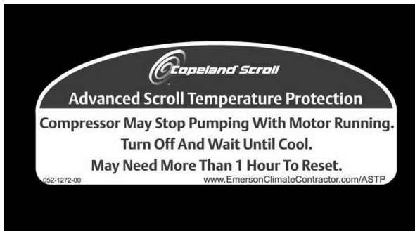
Fig. 14 - Advanced Scroll Temperature Protection Label
