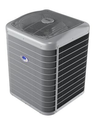
Carrier's 27VNA1 Cold Climate Heat Pump with Greenspeed™ Intelligence is another breakthrough product providing up to 12.5 HSPF2 heating efficiency and up to 21 SEER2 cooling efficiency. The variable speed capacity control achieves 100% heating capacity down to 5°F. Lower speed operation is available when needed in cooling for enhanced comfort and dehumidification.
